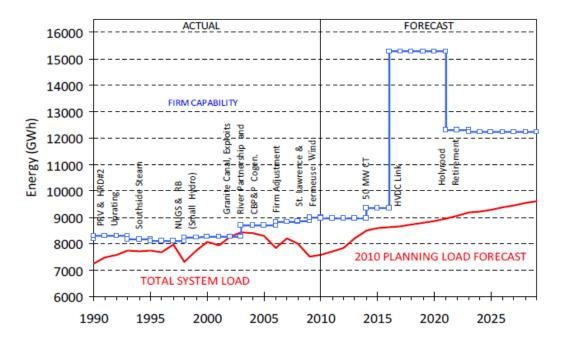
Preliminary HVdc Link Expansion Plan vs. Load Forecast
