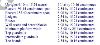
(2) Components of double-pole scaffolds shall have minimum nominal dimensions conforming to the following table:
