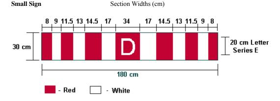
If a lighted sign box is used, it must meet the following specifications:
