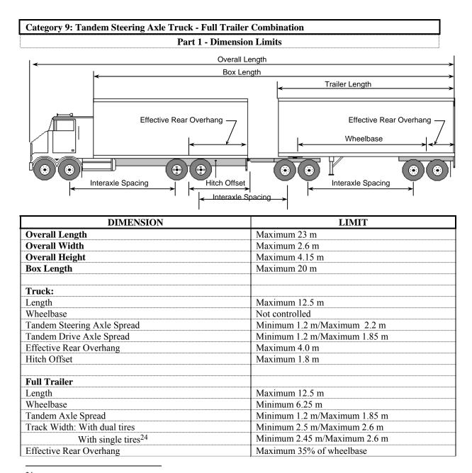
$^{24}$  The minimum track width for trailers fitted with single tires and manufactured prior to 2010 is 2.3 metres.
