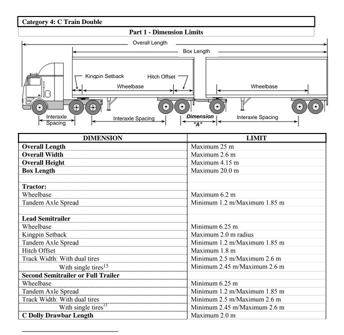
$<sup>^{15}</sup>$  The minimum track width for trailers fitted with single tires and manufactured prior to 2010 is 2.3 metres.
