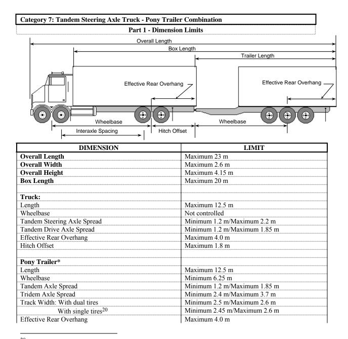
$<sup>^{20}</sup>$  The minimum track width for trailers fitted with single tires and manufactured prior to 2010 is 2.3 metres.
