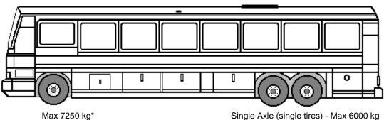
Single Axle (dual tires) - Max 9100 kg Tandem Axle - Max 18 000 kg
