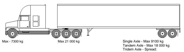
2.4 m to < 3.0 m - Max 21 000 kg 3.0 m to < 3.6 m - Max 24 000 kg 3.6 m to 3.7 m - Max 26 000 kg
