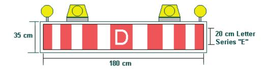
**Box Dimensions** - the box must be 180 centimetres x 35 centimetres x 10 centimetres and constructed of mild steel material with inside and outside surfaces of baked white enamel. The box must shelter all wire connectors, switches, flashers, etc.
