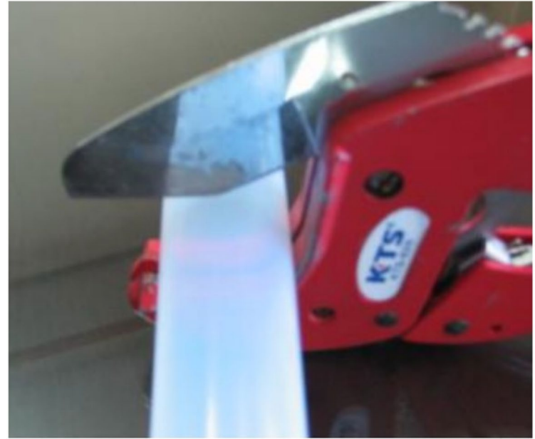
Figure 3: Cutting the tube square
