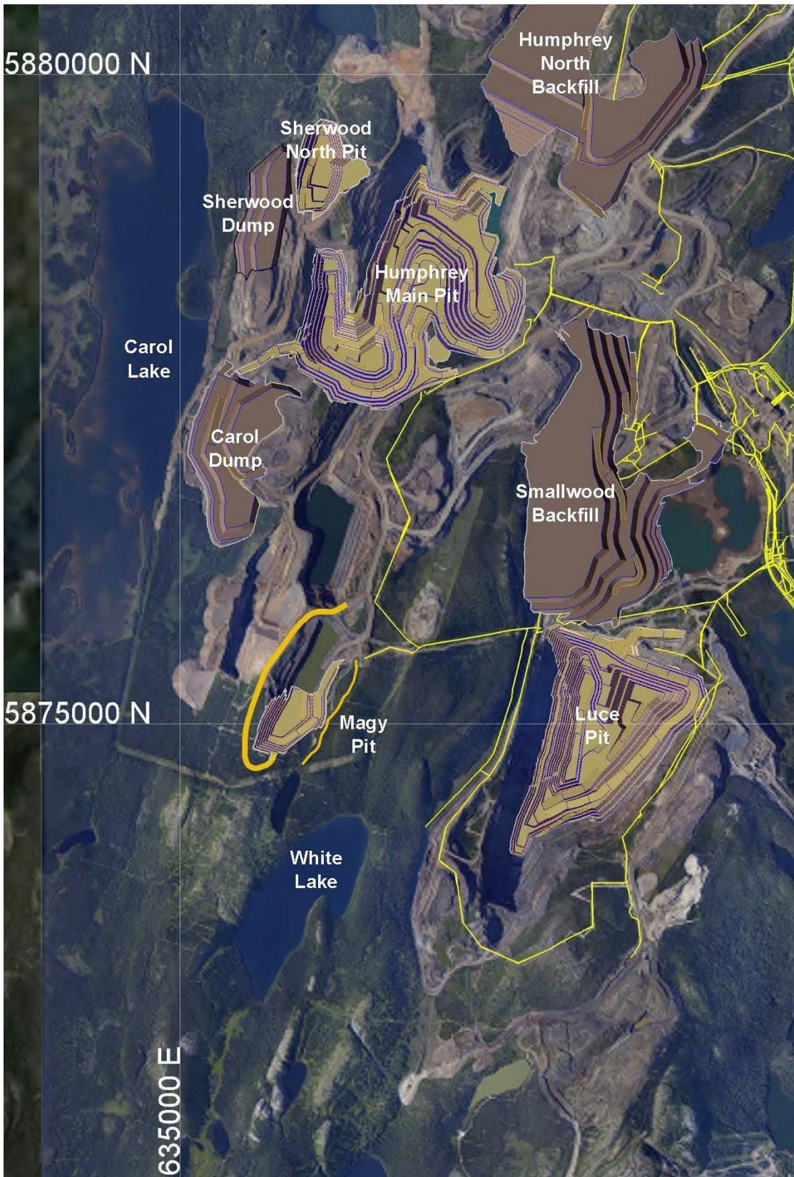
Figure 7: Mine Configuration after Completion of Luce, Humphrey Main and Magy Pits
