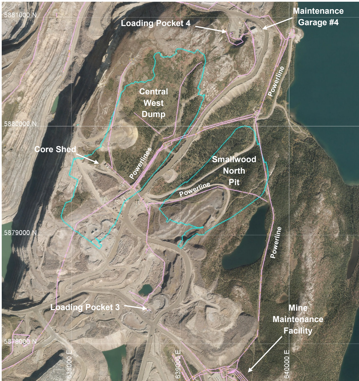
Figure 10: Power Line Network
