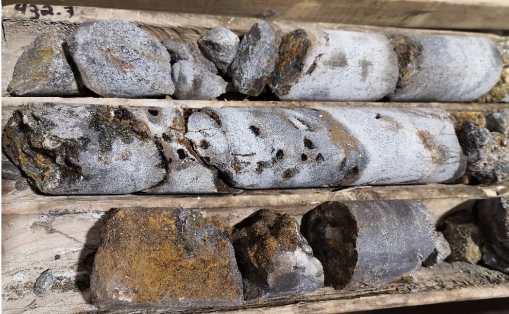
Figure 2-2: Vuggy Bedrock Located at Around 430 m in the Sokoman Formation (KGT-23-03)
