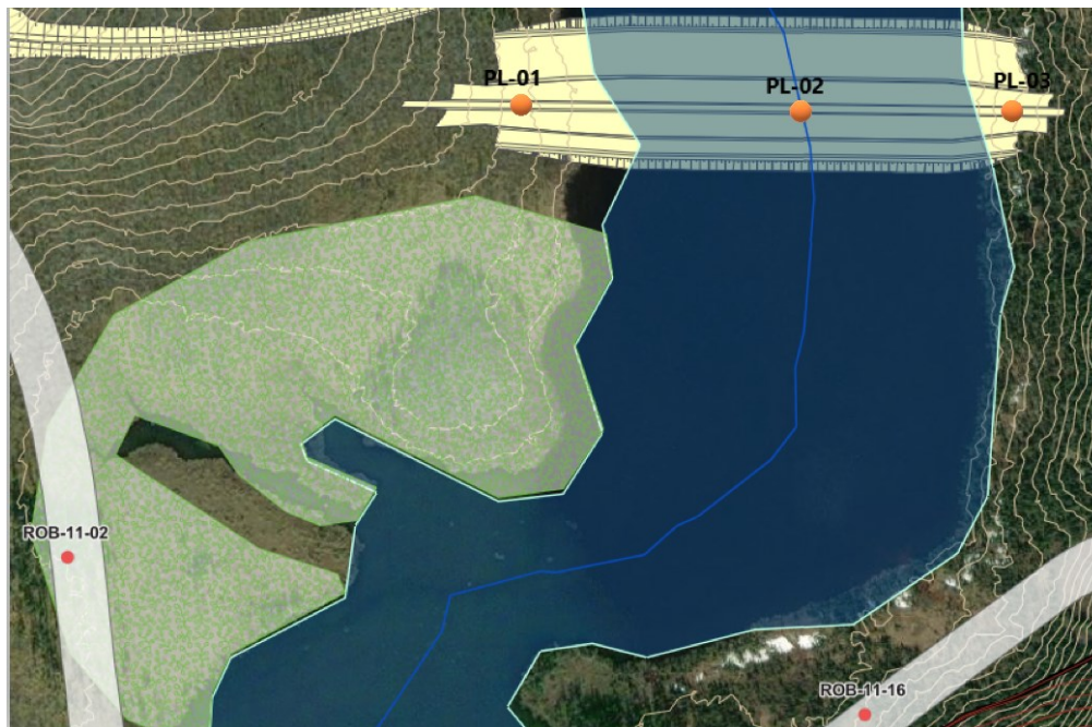
Figure I-5: Proposed Boreholes for Pike Dike
