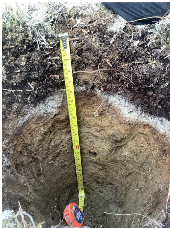
Photo C-12: Eluviated Dystric Brunisol (E.DYB) pit profile at plot K23LM023. Till material, example of material for Labrador (LAB) SMU. 26 September 2023
