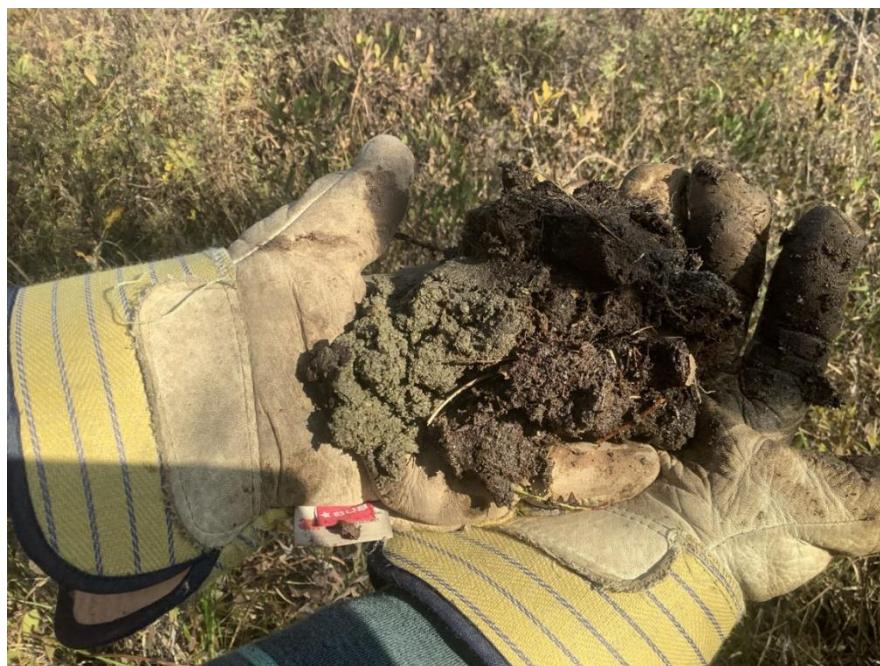
Photo C-16: Terric Mesisol (T.M) material profile at plot K23CB024. Mesic organic material and coarse fragments, example of material for Mills Lake (MIL) SMU. 28 September 2023
