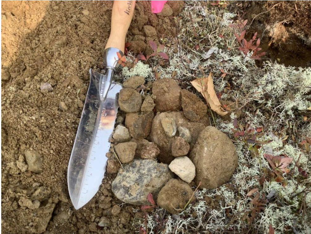
Photo C-13: Example of coarse fragments from plot K23LM010. Till material, example of material for Labrador (LAB) SMU. 26 September 2023
