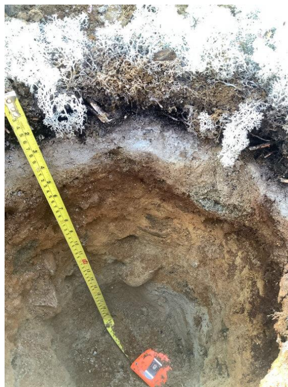
Photo C-10: Orthic Humo Ferric Podzol (O.HFP) pit profile at plot K23CB023. Till material, example of material for Javelin Road (JAV) SMU. 28 September 2023
