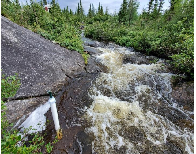
Photograph 70: WC-07 staff gauge; view looking southeast and downstream on August 10, 2023.
