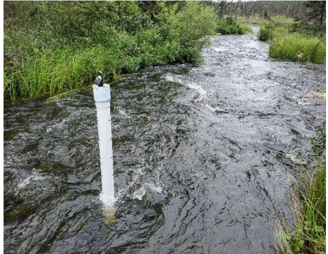
Photograph 2: WC-02 staff gauge; view looking north and downstream on August 11, 2023.
