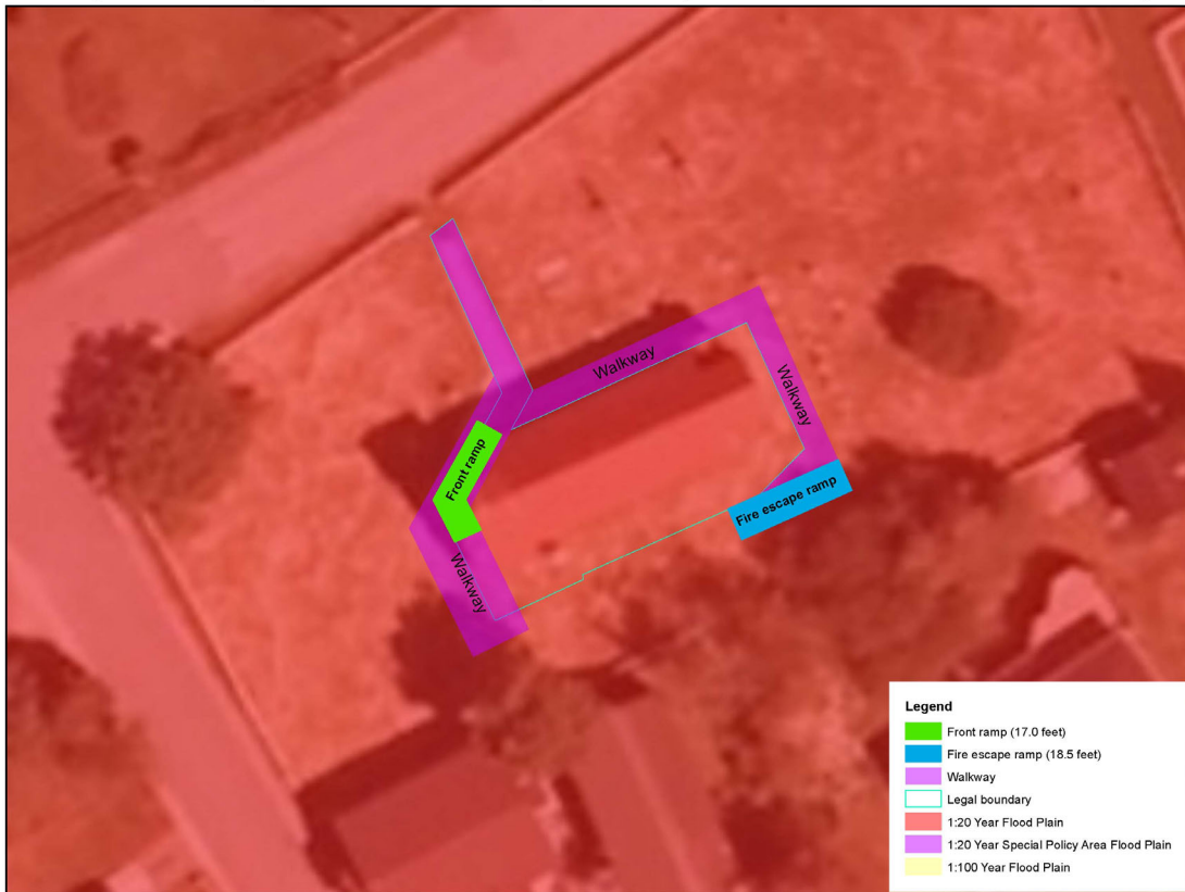
Ramp and walkway construction on a designated flood plain at Placentia Area Historical Society
