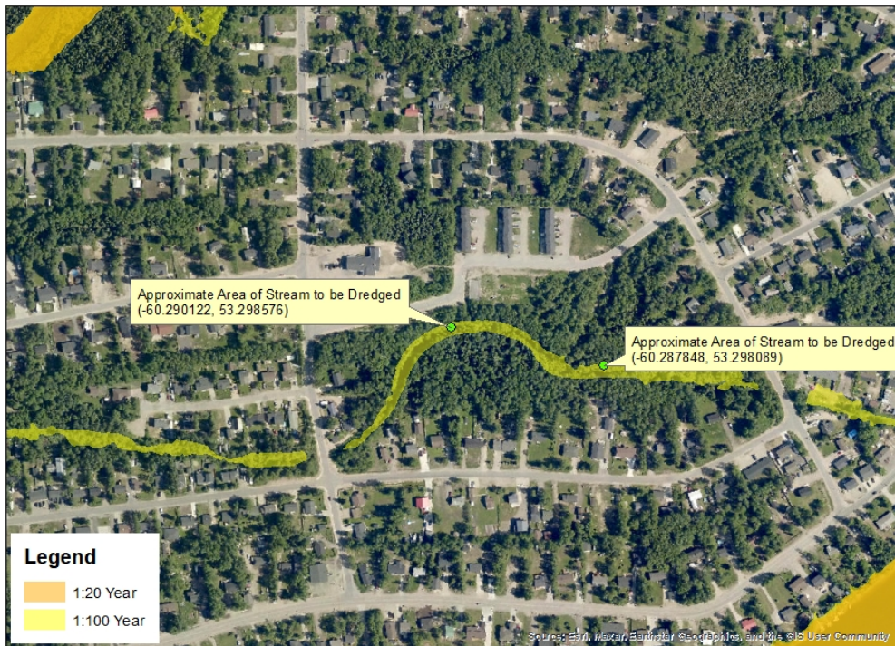
Dredging and Cleaning of an Unnamed Stream near Cartwright Road, Happy Valley - Goose Bay
