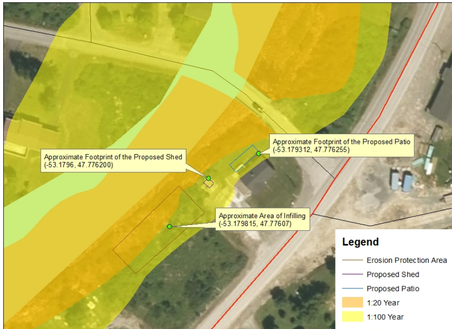
Work within the Designated Flood Plain in the Town of Salmon Cove
