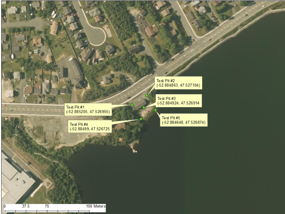
Geotechnical Test Pits in the Town of Paradise
