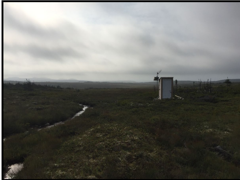
Figure 4: Real-Time Water Quality and Quantity Station at Outflow of Unnamed Pond south of Long Pond
