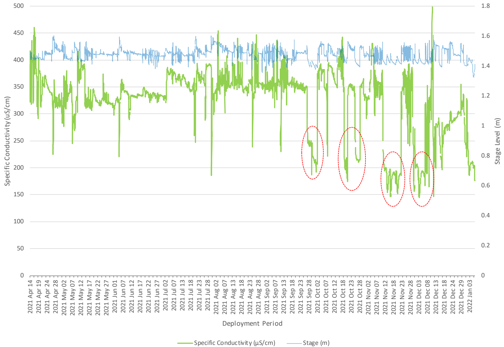
Specific Conductivity ( \mu\text{S}/\text{cm} ) and Stage level (m) recorded at Outflow of Grebes Nest Pond
