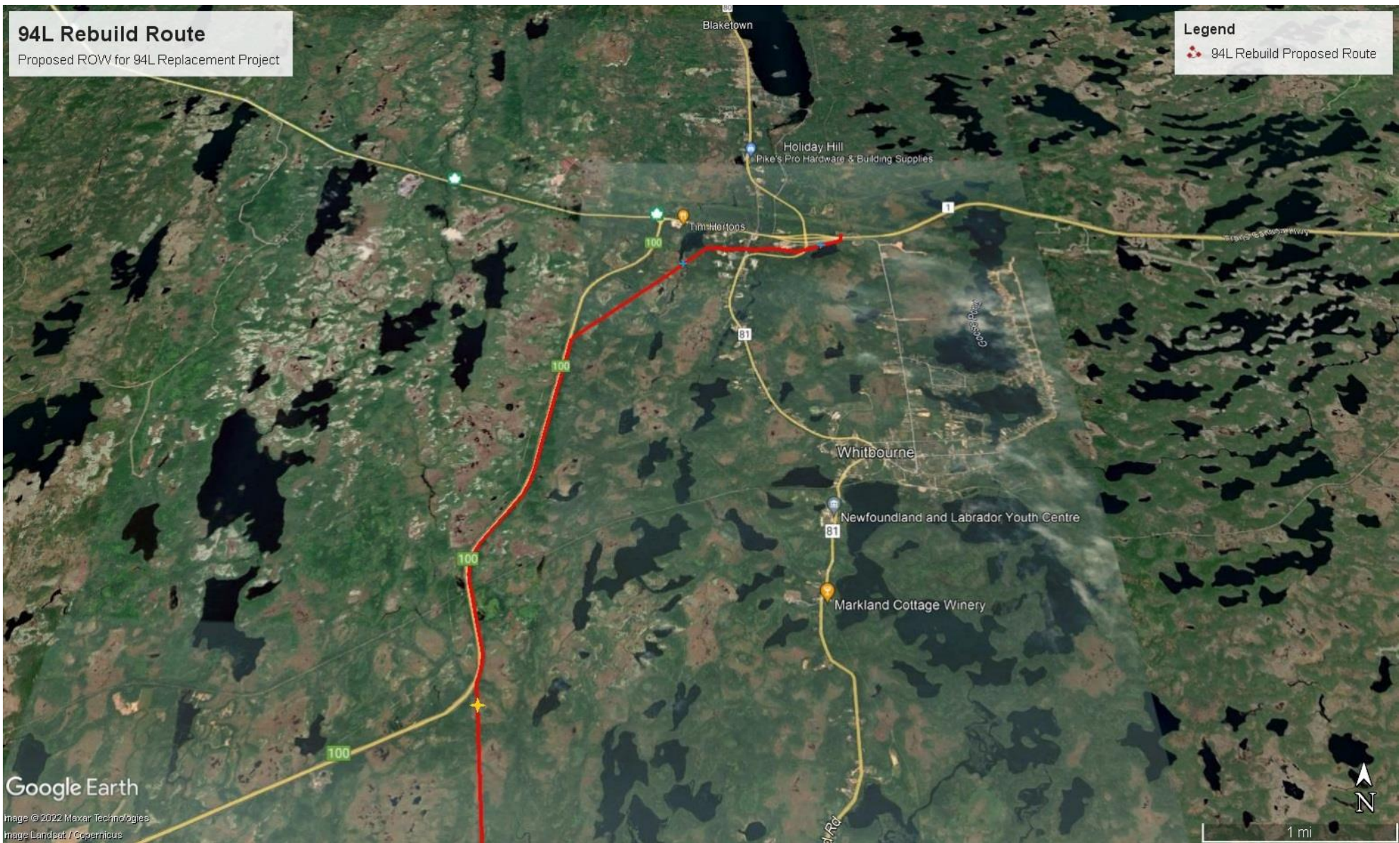
Figure B-8: Phase 3 (2024) completing line from halfway point to Blaketown Substation. Crossing sites of rivers identified on 1:50 000 mapping are identified by a blue marker. Crossings of Salmon rivers and tributaries identified on 1:50 000 mapping are identified by a yellow marker.
