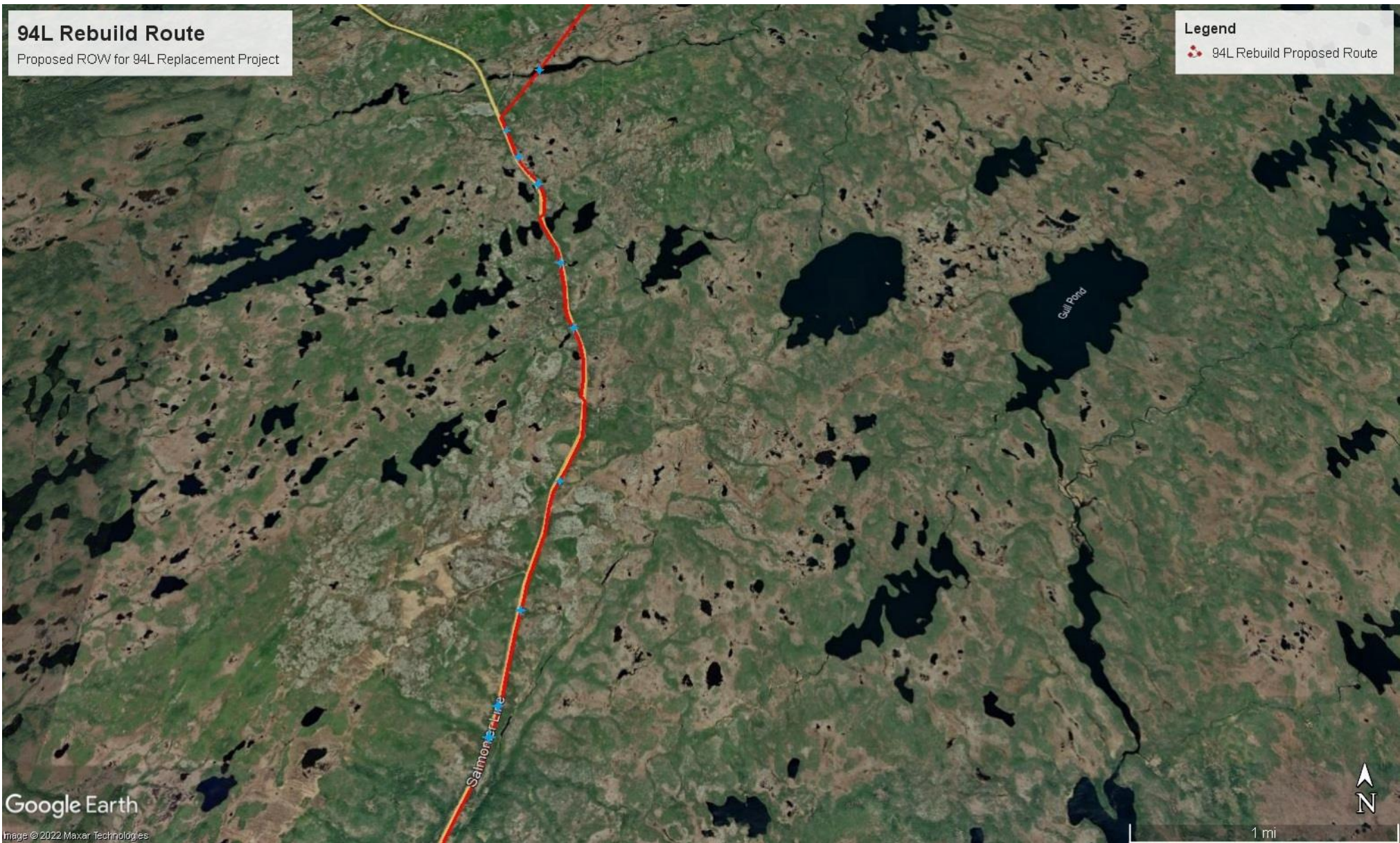
Figure B-3: Phase 1 (2022) extending from Riverhead Substation to St. Catherine's Substation. Crossing sites of rivers identified on 1:50 000 mapping are identified by a blue marker. Crossings of Salmon rivers and tributaries identified on 1:50 000 mapping are identified by a yellow marker.
