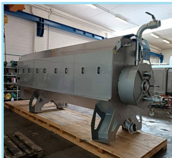
SD SLUDGE PRESS READY FOR SHIPMENT
