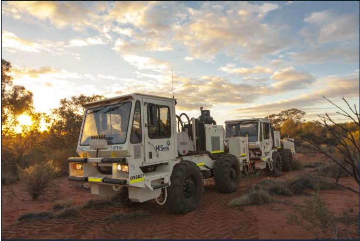
Photo 1: HiSeis Energy Source Thumper Truck (Vibroseis) with Low-Impact Tires
