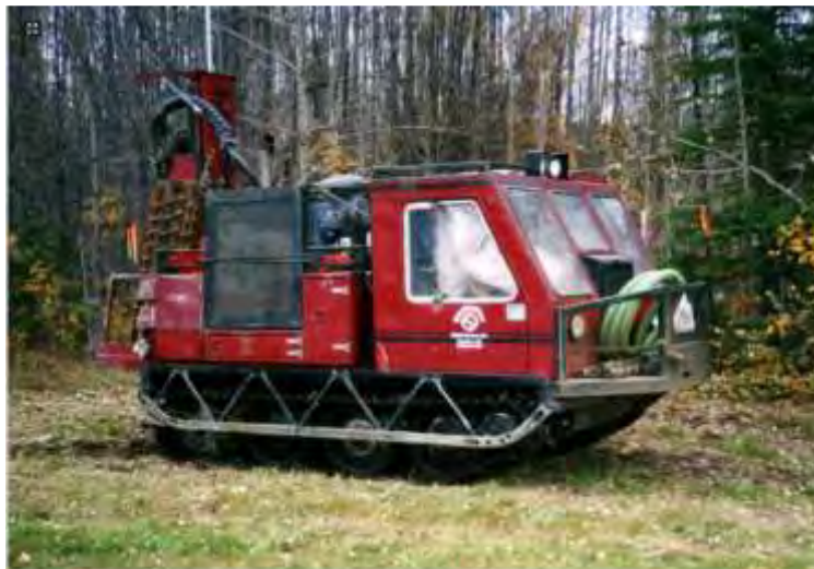
Photo 2: Overburden (Auger) Drill for Seismic Charge Energy Source boreholes
