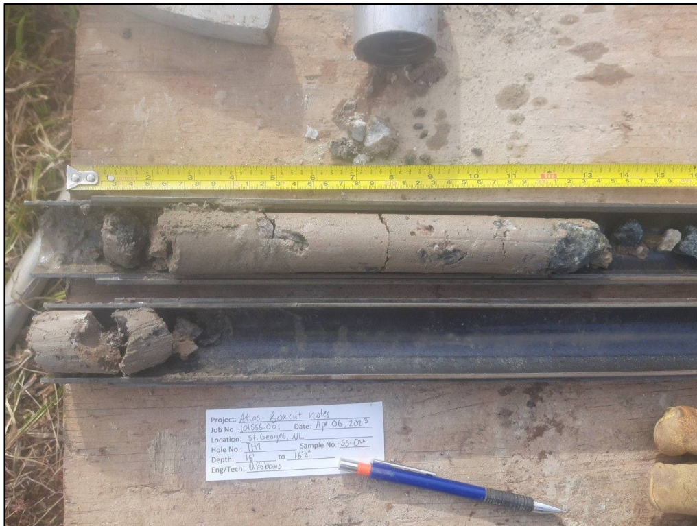
Figure TH1.4 TH1 split spoon sample SS4 from 4.57 m to 4.93 m
