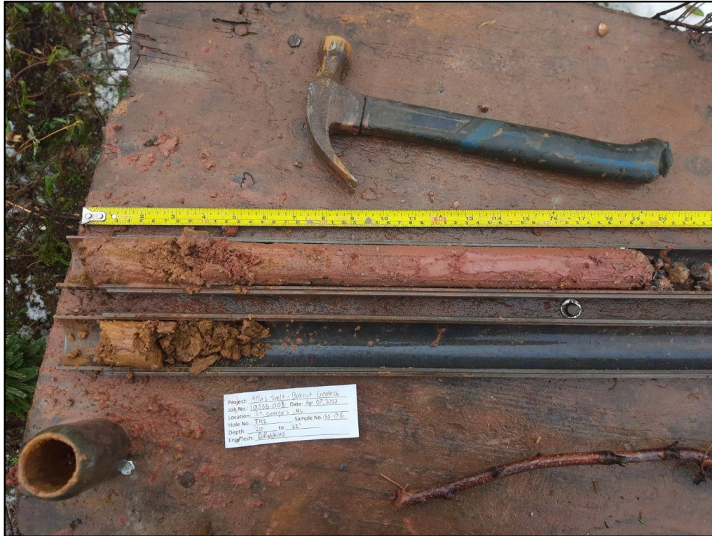
Figure TH2.5 TH2 split spoon sample SS5 from 6.10 m to 6.71 m
