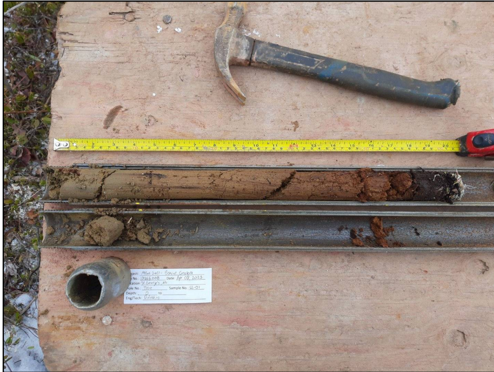
Figure TH4.1 TH4 split spoon sample SS1 from 0 m to 0.61 m
