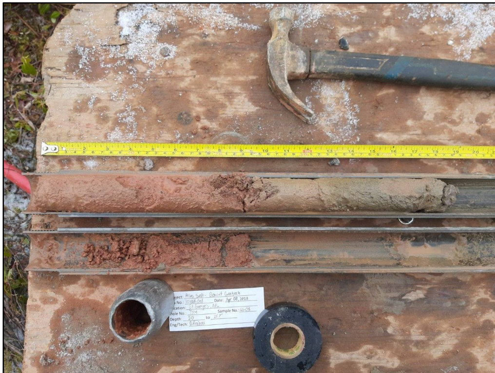
Figure TH4.4 TH4 split spoon sample SS5 from 6.10 m to 6.58 m
