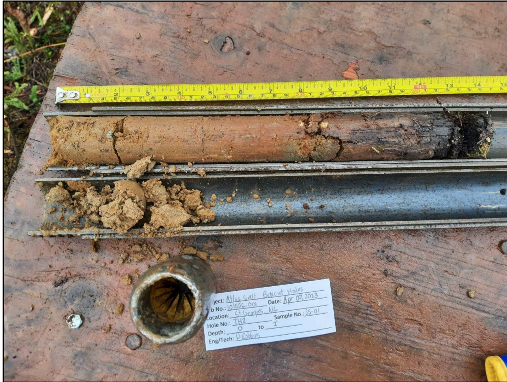
Figure TH2.1 TH2 split spoon sample SS1 from 0 m to 0.61 m
