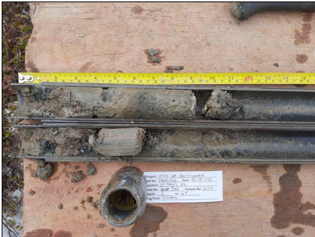
Figure TH4.2 TH4 split spoon sample SS2 from 1.52 m to 2.06 m
