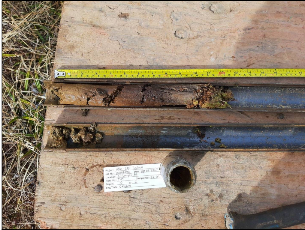
Figure TH1.1 TH1 split spoon sample SS1 from 0 m to 0.61 m
