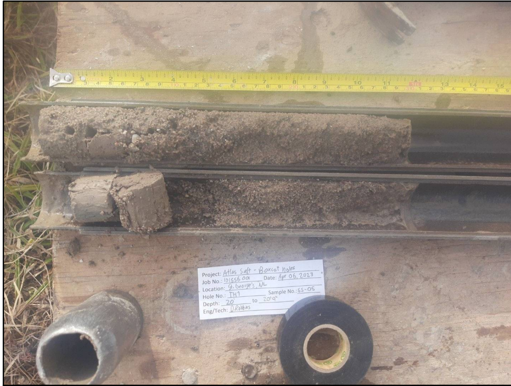
Figure TH1.5 TH1 split spoon sample SS5 from 6.10 m to 6.32 m
