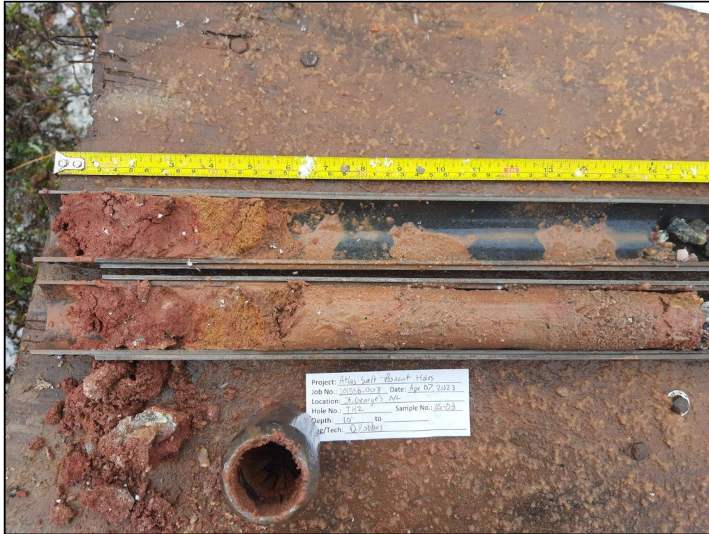
Figure TH2.3 TH2 split spoon sample SS3 from 3.05 m to 3.66 m
