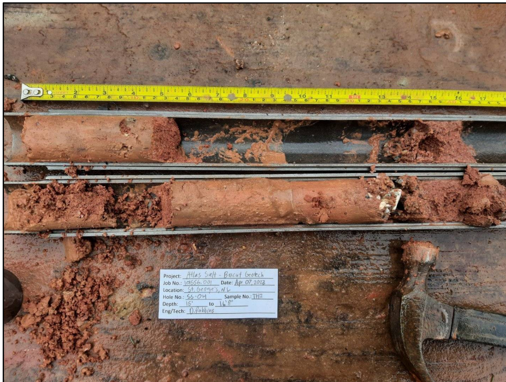
Figure TH2.4 TH2 split spoon sample SS4 from 4.57 m to 5.08 m
