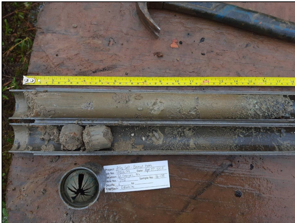
Figure TH2.2 TH2 split spoon sample SS2 from 1.52 m to 2.13 m
