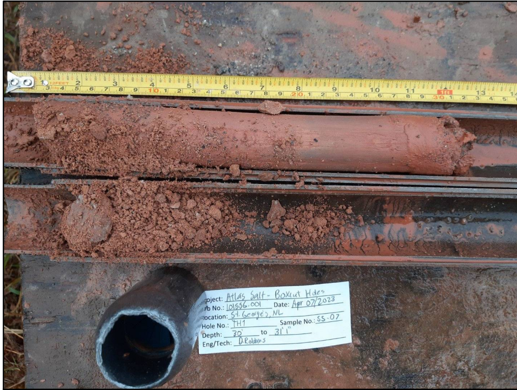
Figure TH1.7 TH1 split spoon sample SS7 from 9.14 m to 9.47 m
