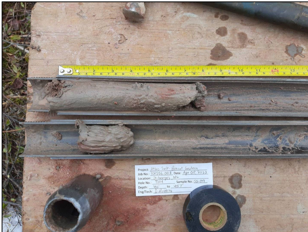
Figure TH4.6 TH4 split spoon from 40' to 40'7"
