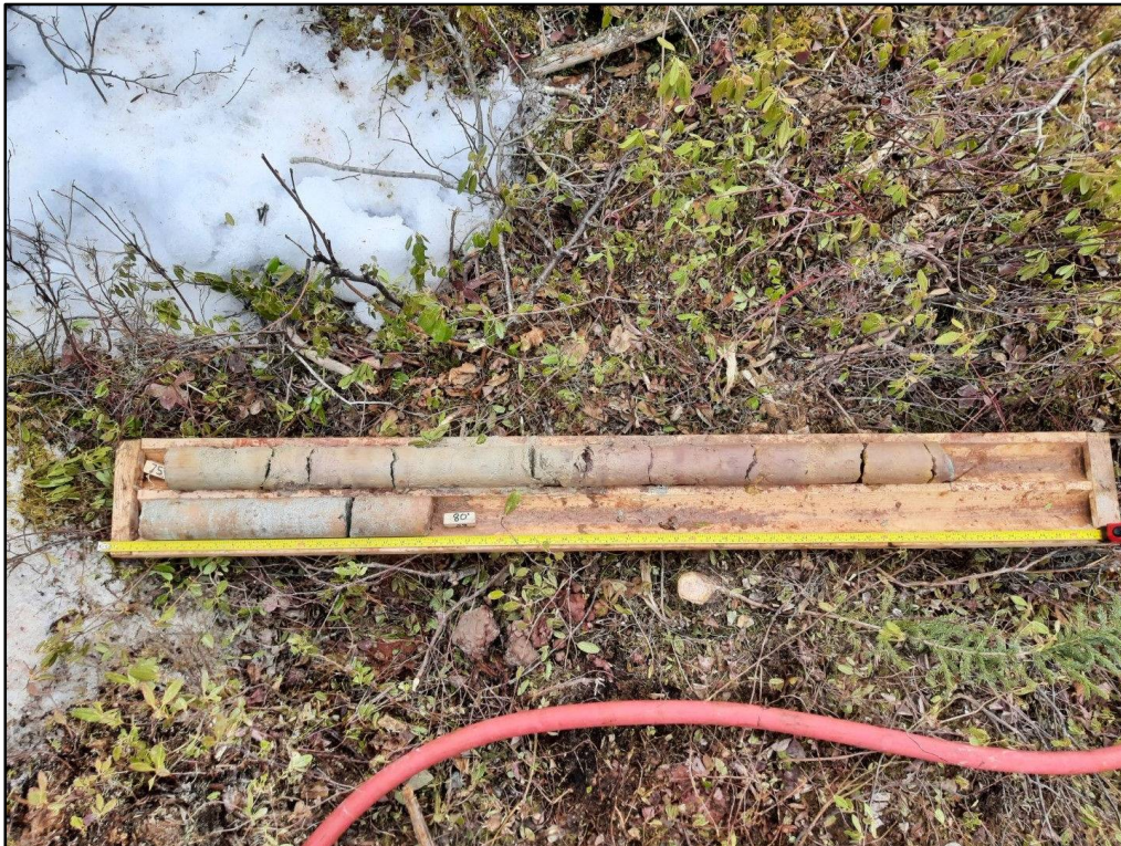
Figure TH4.10 Rock core from 22.86 m to 24.38 m
