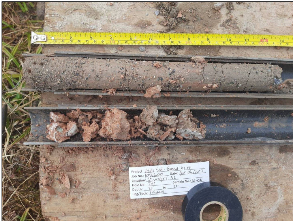
Figure TH1.6 TH1 split spoon sample SS6 from 7.62 m to 8.23 m
