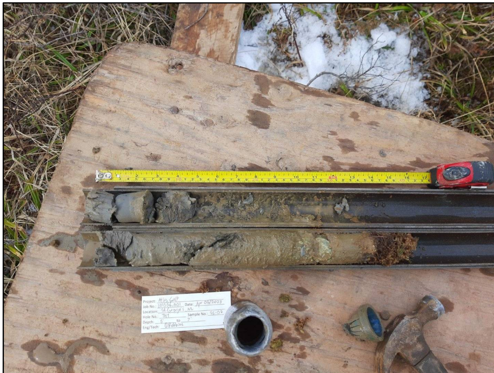
Figure TH1.2 TH1 split spoon sample SS2 from 1.52 m to 2.13 m
