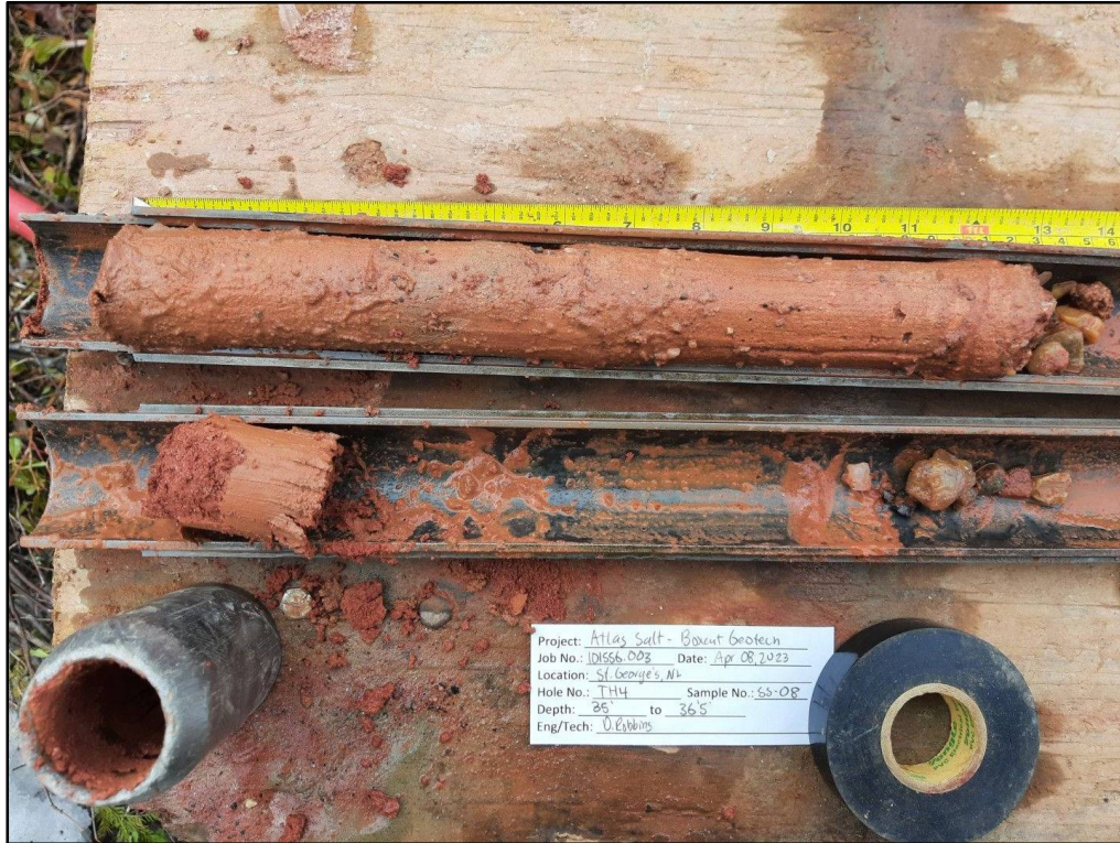
Figure TH4.5 TH4 split spoon sample SS8 from 10.67 m to 11.10 m
