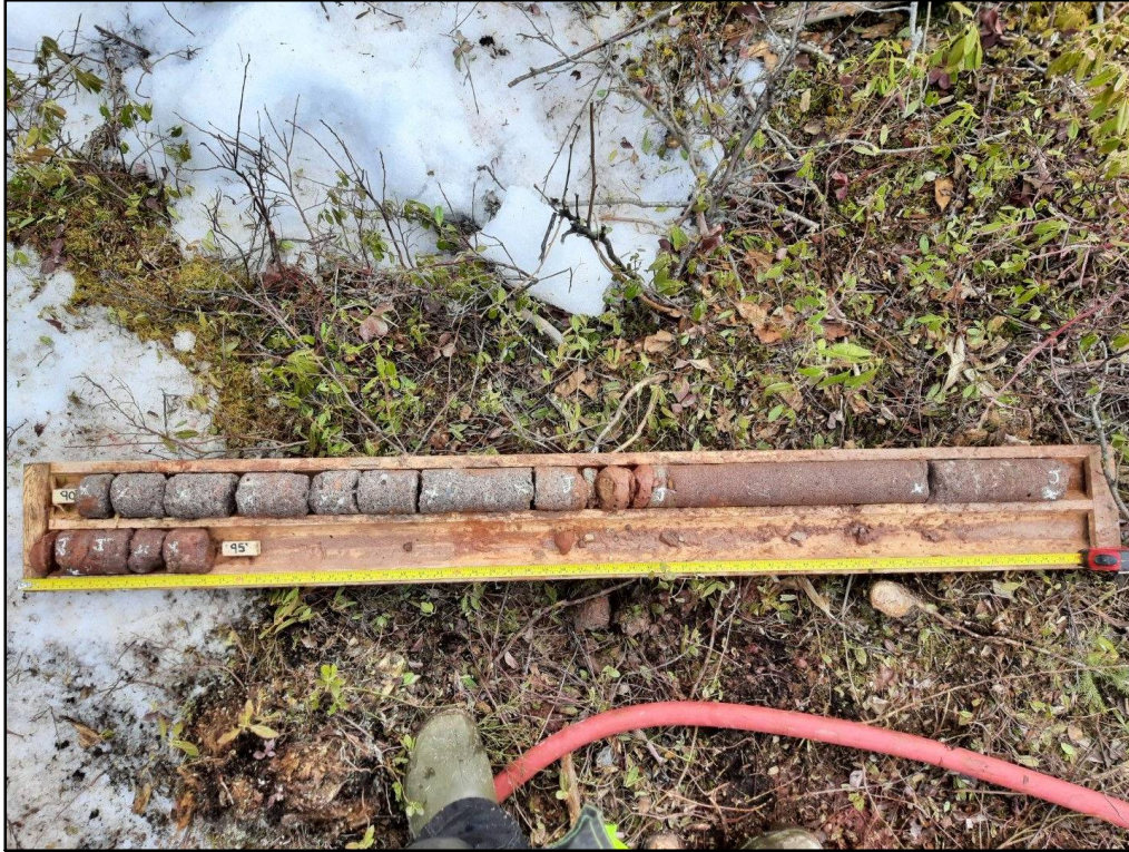
Figure TH4.13 Rock core from 27.43 m to 28.96 m
