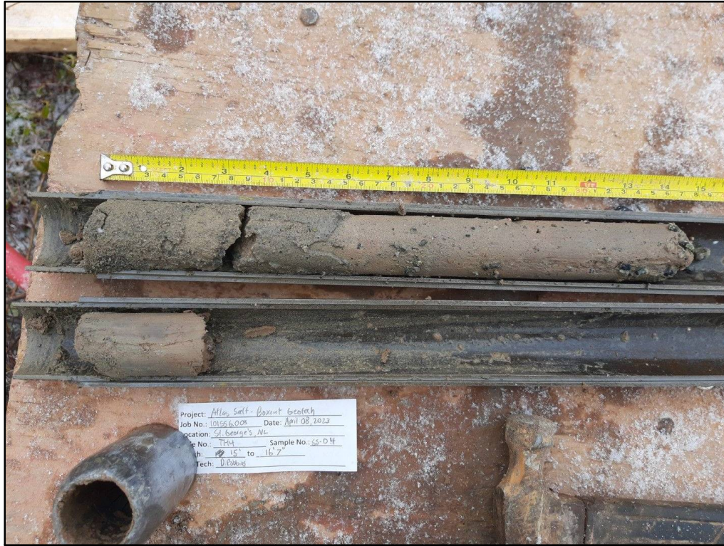
Figure TH4.3 TH4 split spoon sample SS4 from 4.57 m to 5.05 m
