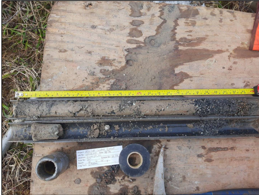
Figure TH1.3 TH1 split spoon sample SS3 from 3.05 m to 3.66 m
