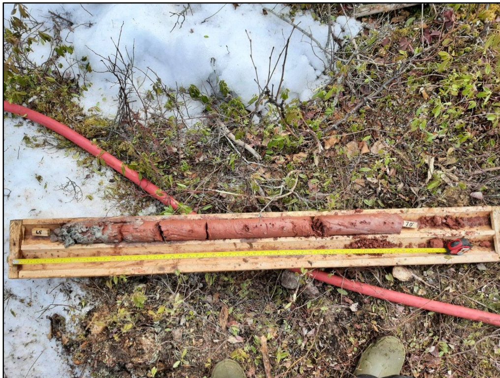
Figure TH4.8 Rock core from 19.81 m to 21.34 m
