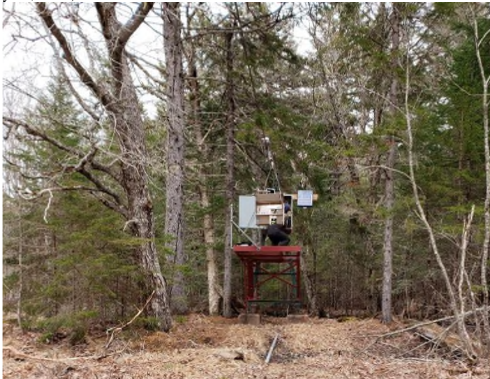
Figure 34. View of the A-frame on the right bank of Kelley River showing the inactive cablecar and the temporary gauge (photograph taken April 23, 2021).
