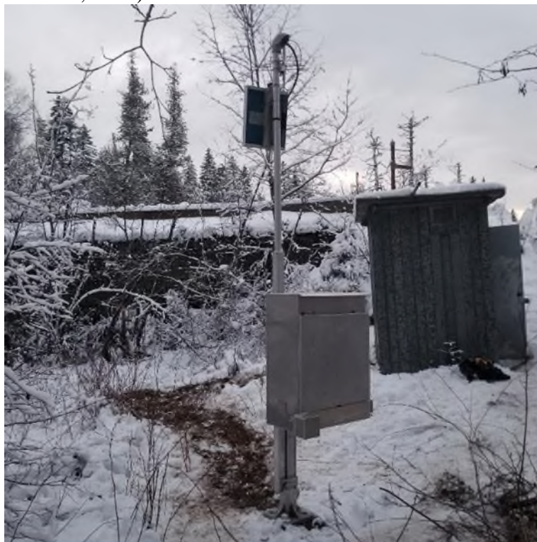
Figure 4. New tilting mast and cabinet at 01BP002 Catamaran Brook at Repap Road Bridge (Photograph taken December 7, 2020).
