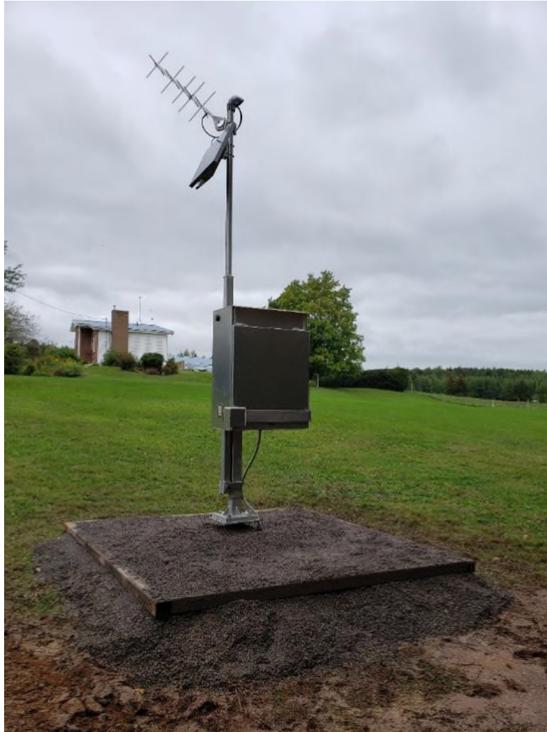
Figure 41. New look-in shelter housing the pressure system at 01DP004 (photograph taken September 29, 2021).
