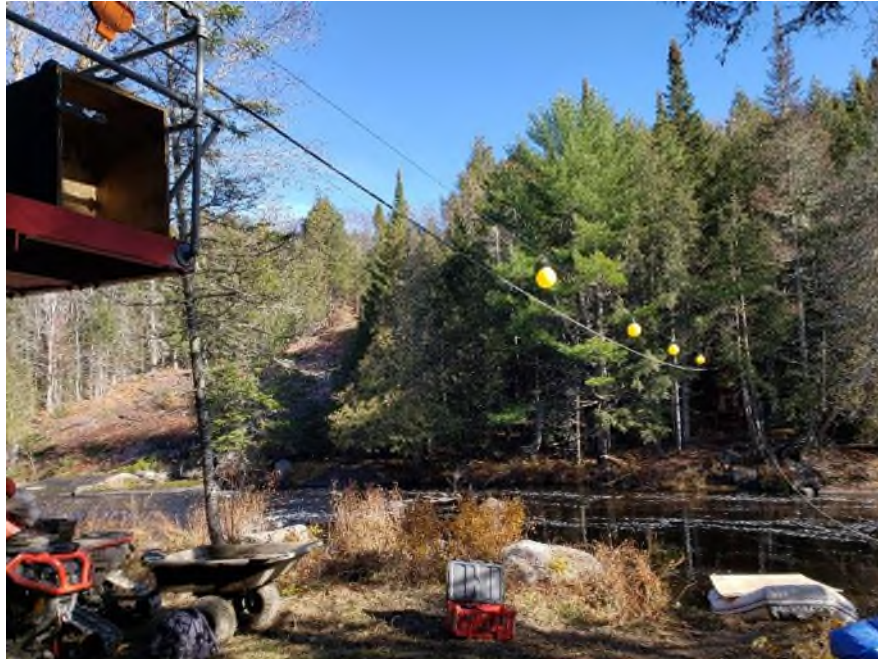
Figure 22. Barossa double drum winch bank-operated cableway at 01AK001 Shogomoc Stream near Trans Canada (Photograph November 4, 2021).
