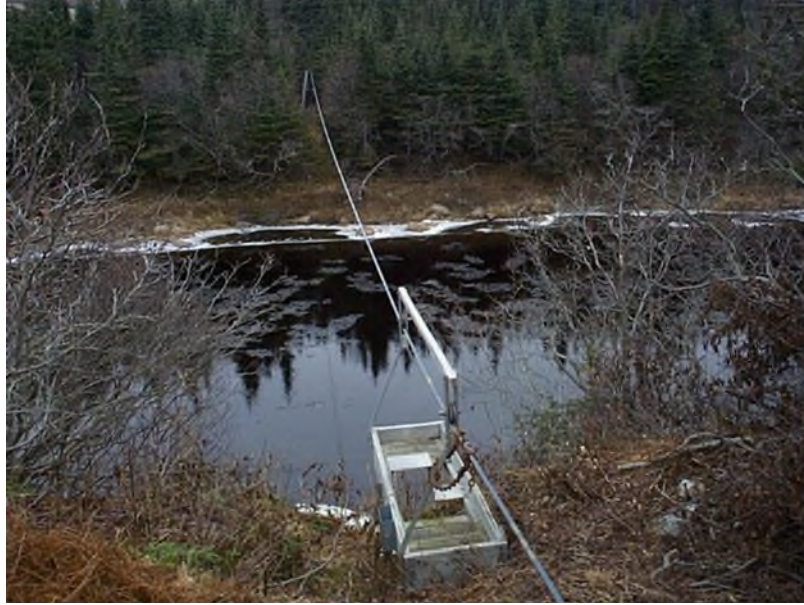
Figure 51. Inactive manned cableway located at 02ZB001 Isle aux Morts below Highway Bridge (Photograph taken November 21, 2007).
