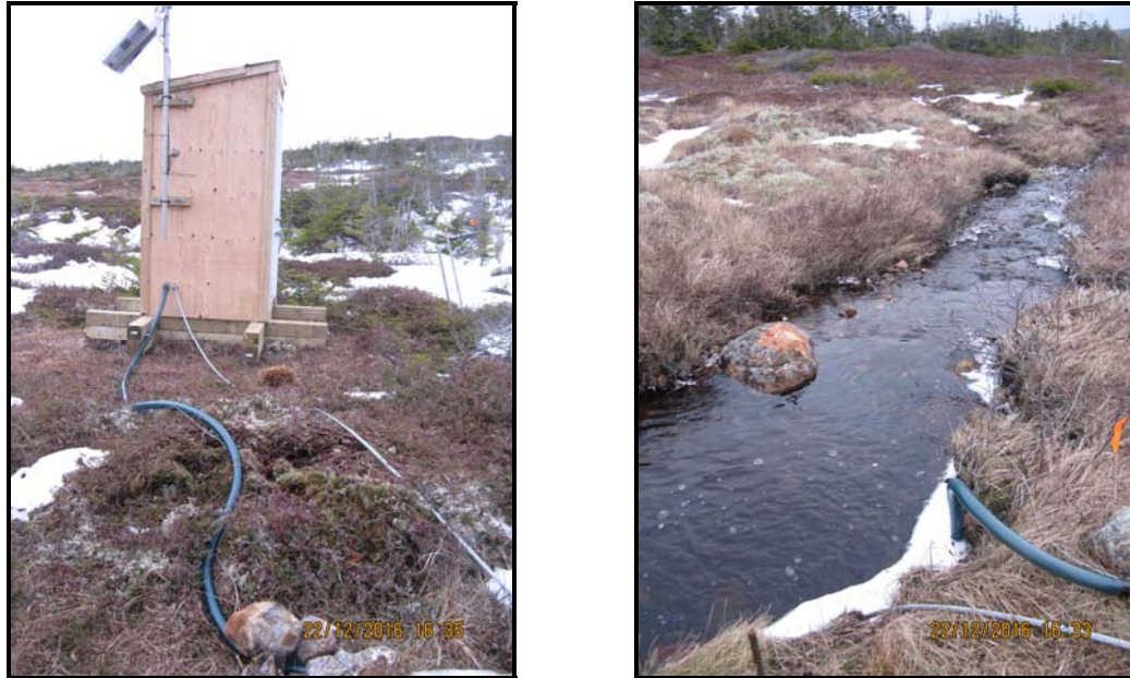
Figure 3: Real-Time Water Quality and Quantity Station at Outflow of Unnamed Pond south of Long Pond.
