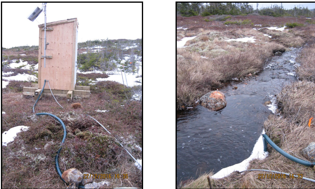
Figure 2: Real-Time Water Quality and Quantity Station at Outflow of Unnamed Pond south of Long Pond.
