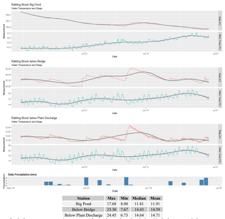
Gradual water temperature increases are observed at each station during this deployment period.
