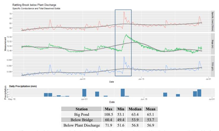
• Specific conductivity was relatively stable at all stations during this deployment period with few fluctuations due to variations in Stage caused by precipitation. There are increases at Big Pond not related to precipitation. This may be due to wave action from the pond occasionally stirring up sediment around the sonde, increasing the conductivity.
