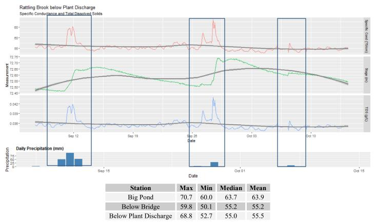
• Specific conductivity was relatively stable at all stations with most peaks occurring during precipitation events. There are increases at Big Pond not related to precipitation. This may be due to wave action from the pond occasionally stirring up sediment around the sonde, increasing the conductivity.
