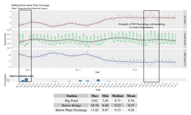
During this time of year, it is expected to find dissolved oxygen concentrations lower than the CCME guideline of 9.5 mg/l for the protection of cold water biota. Cooler water temperatures mid deployment period allowed oxygen concentrations to rise at all stations.
