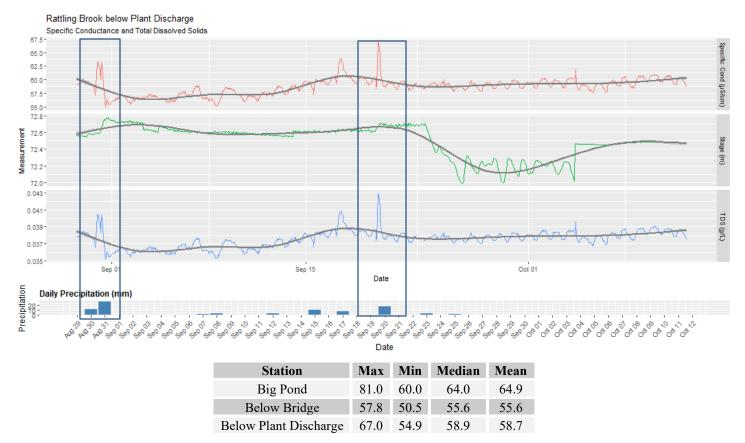
Specific conductivity was relatively stable at all stations with most peaks occurring during precipitation events.
