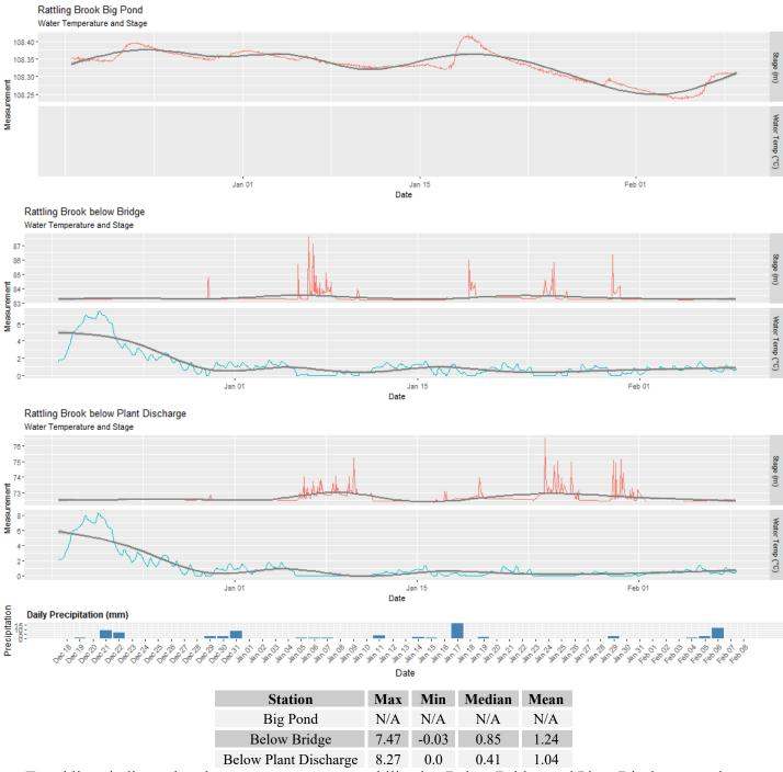
Trend lines indicate that the water temperature stabilized at Below Bridge and Plant Discharge stations.
