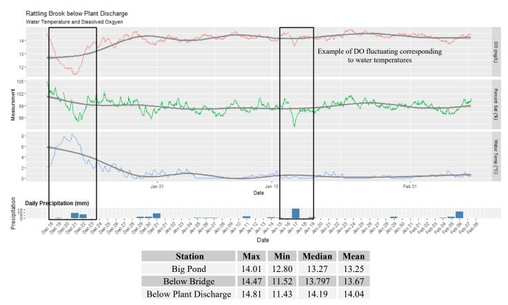
• As shown on all three graphs, DO is slowing increasing at all three stations as water temperatures cool. This aligns with the CCME guideline of 9.5 mg/l for the protection of cold water biota.
