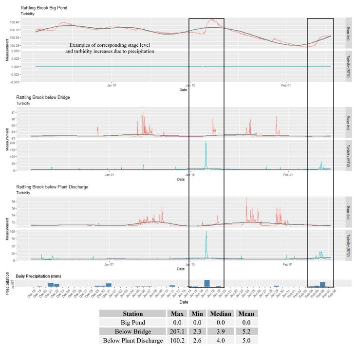
• Big Pond is ice covered hence the 0.0NTU readings as sediment isn't moving around without wave action. Turbidity was stable at Below Bridge and Plant Discharge with exception of during precipitation events.
