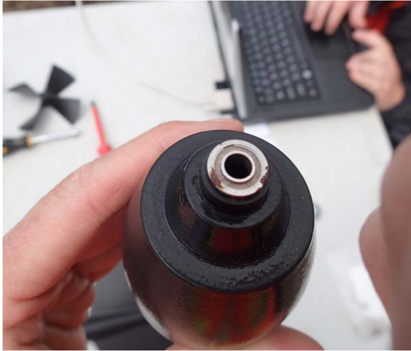
Figure 8: Anemometer bearing corrosion - Upper Humber River above Black Brook
