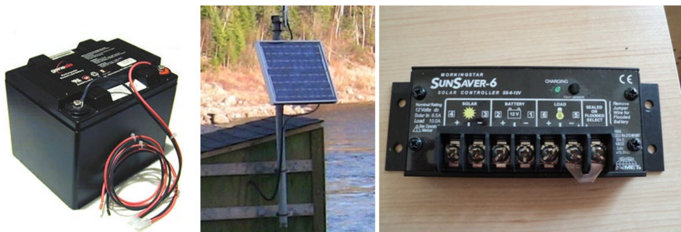
Figure 3-11: (L) 12V Battery to power an RTWQ station; (M) solar panel on an RTWQ Station; (R) Solar power regulator on RTWQ Station
