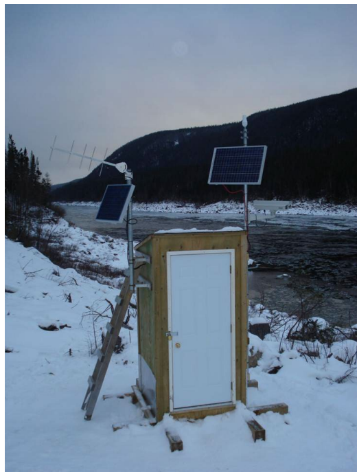
Figure 3-8: RTWQ station with web camera is equipped with iridium satellite for communication in remote areas.
