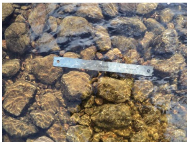
Figure 4-20: (L) Small rocky bed material is best for an RTWQ deployment; (R) Sandy river reaches should be avoided if possible for RTWQ monitoring as sand and silt can cause the sensors to fail
