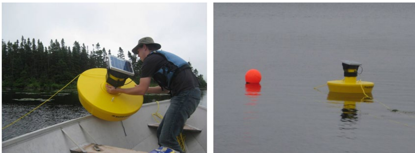
Figure 4-14: Example of a buoy deployment at the Paddy’s Pond NL RTWQ research site
