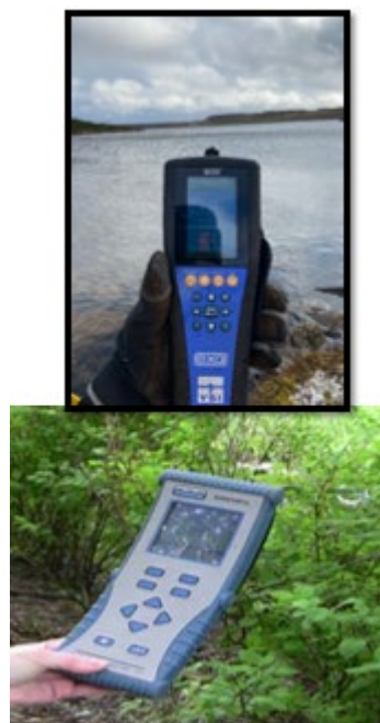
Figure 3-4: Hand held display units for viewing water quality data in-situ
