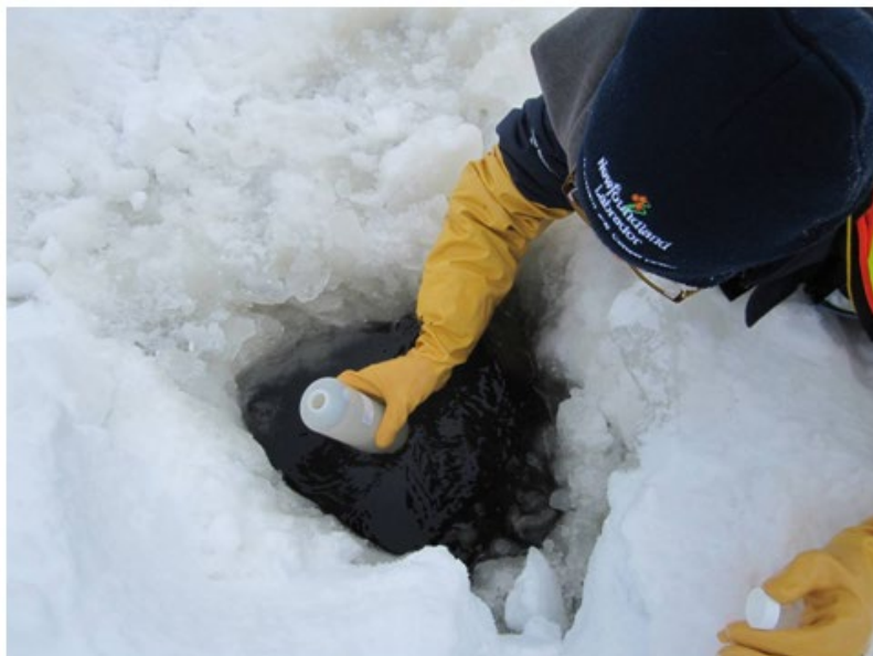
Figure 6-2: (L) Example of grab sample bottles from an accredited laboratory; (R) WRMD takes a RTWQ QAQC grab sample from a hole in the ice
