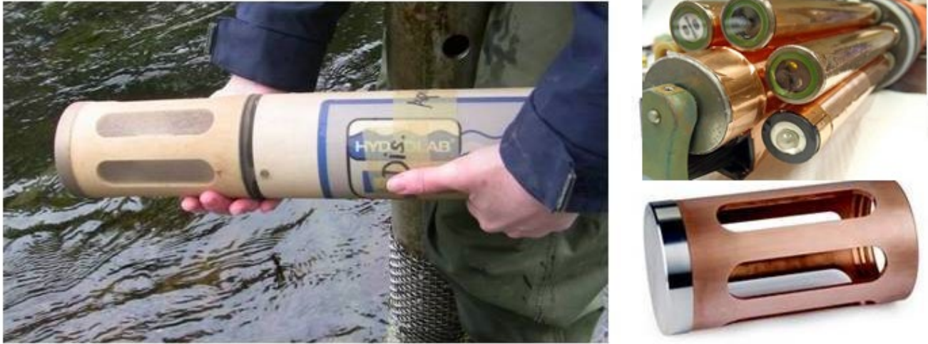
Figure 6-4: (L) Pantyhose used to cover the instrument prior to deployment can sometimes reduce biofouling growth on the instrument (R) Copper plated sensors are sometimes used to reduce the biofouling growth at RTWQ stations
