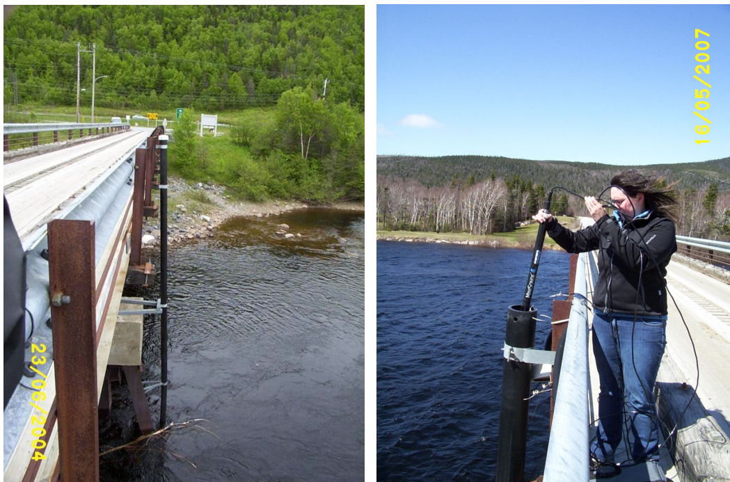
Figure 4-12: Example of a bridge deployment on the Humber River in Western Newfoundland
