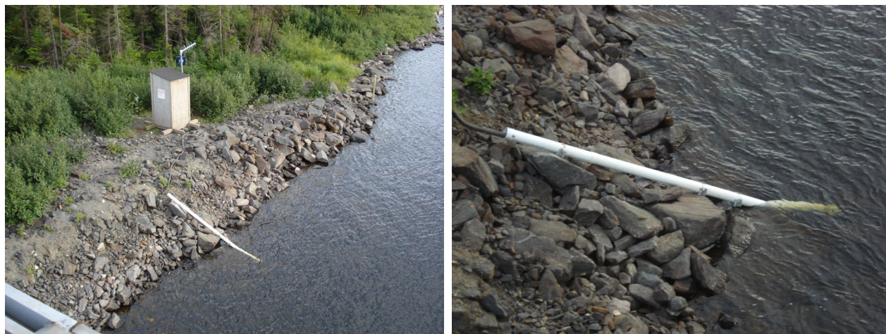
Figure 4-10: Example of shoreline deployments in a river using a pipe
