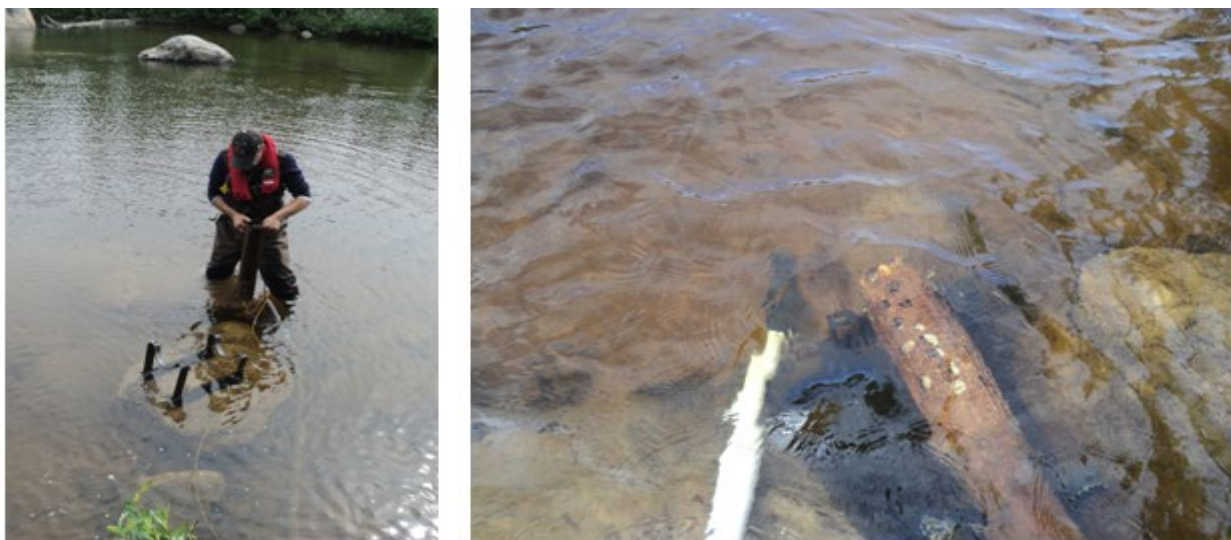
Figure 4-21: A custom built stand was created to hold the instrument off the surface of a sandy river bottom at an RTWQ monitoring station in Labrador
