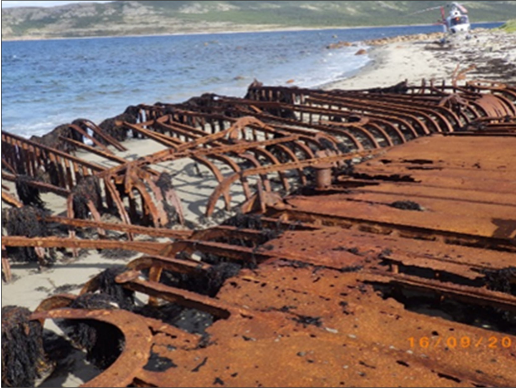
PHOTO 45 - APEC #8: Close-up view of the degraded steel barge on the sandy beach.
