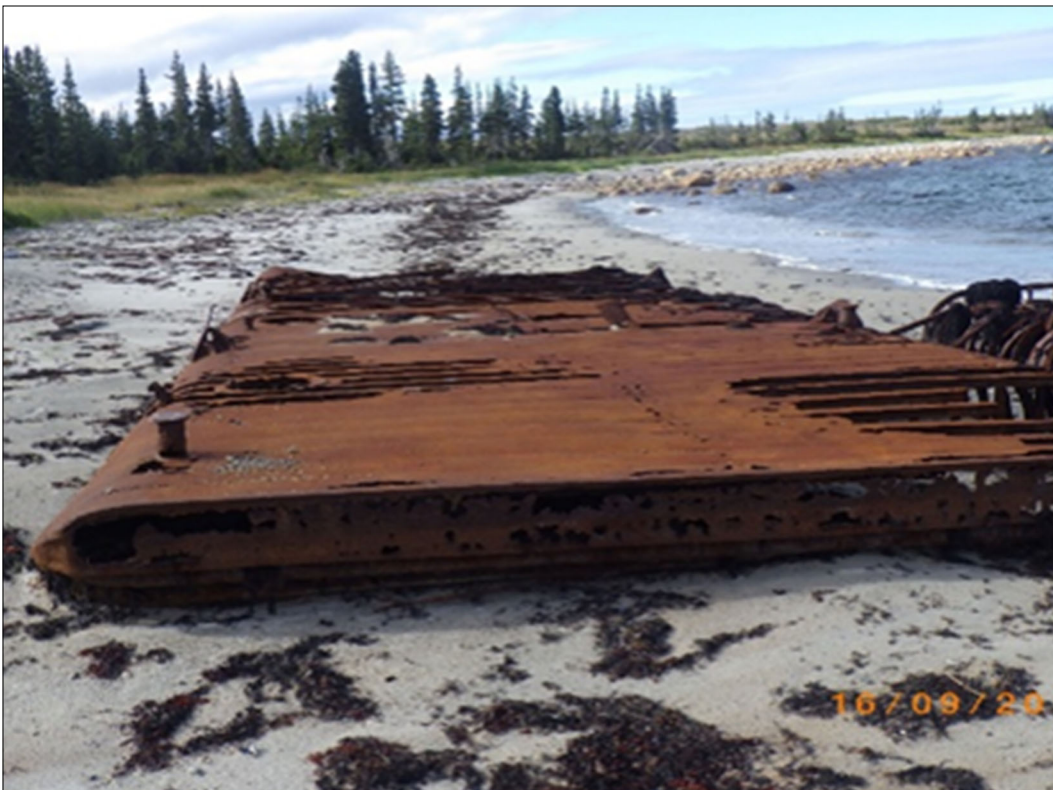
PHOTO 44 - APEC #8: Close-up view of the degraded steel barge on the sandy beach. (September, 2017)
