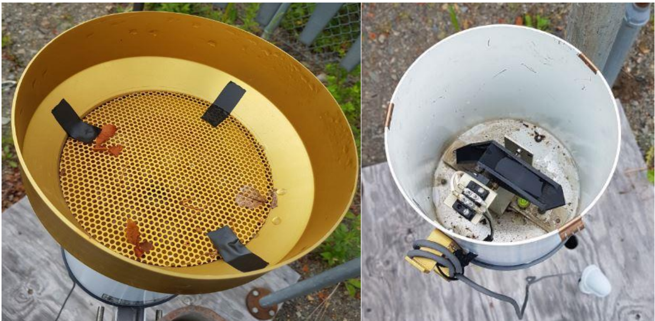
Figure 26: Debris in Tipping Bucket
