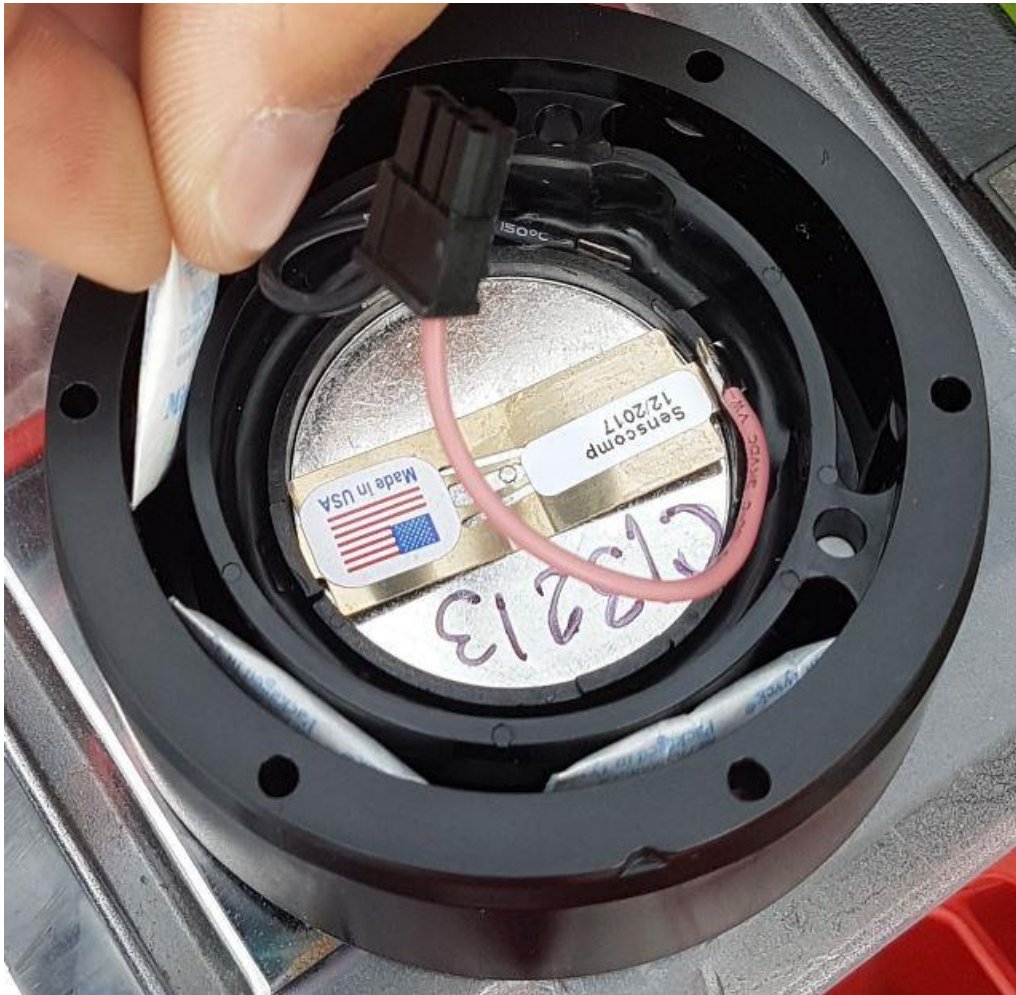
Figure 15: Desiccant Packs Placement
