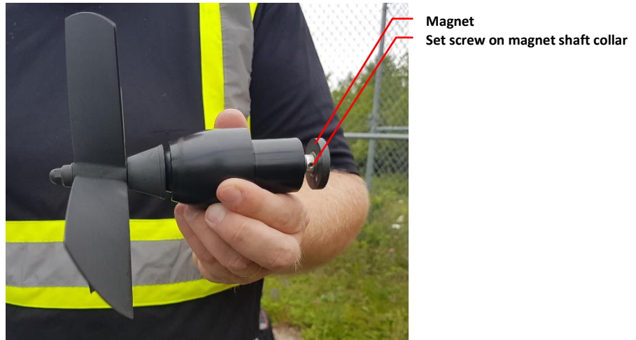
Figure 30: Magnet Set Screw
