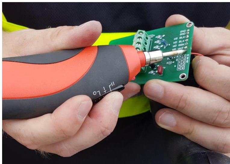
Figure 35: Desoldering PCB Board
