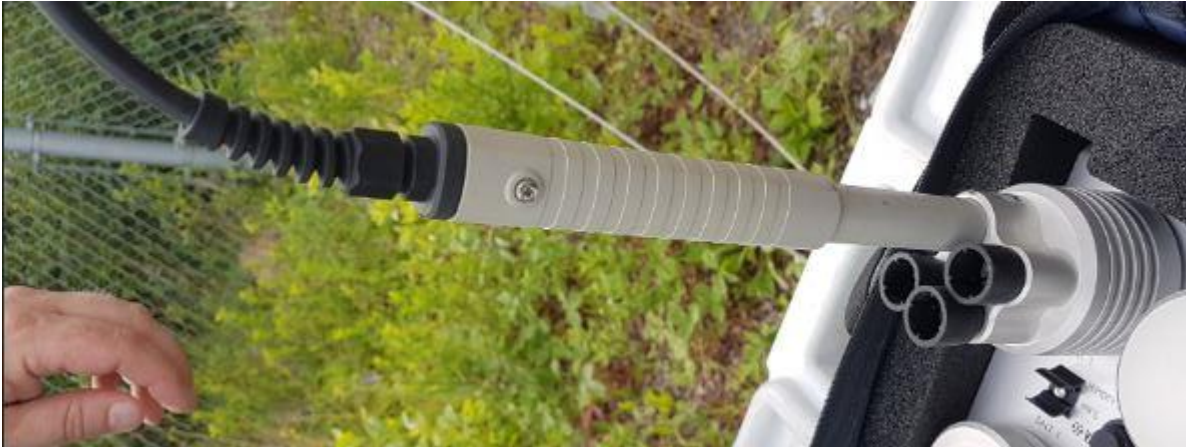
Figure 22: HMP45C Suspended Over LiCl Solution
