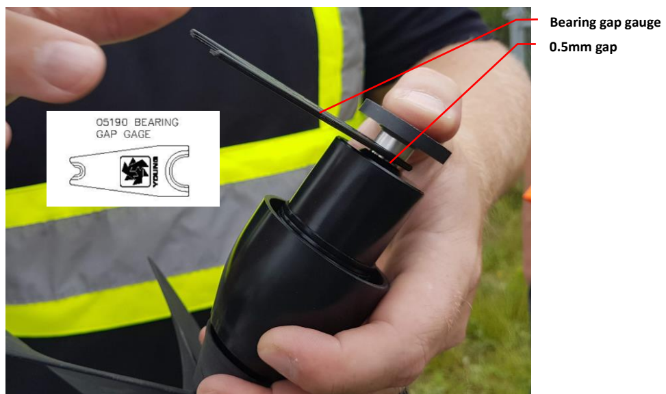
Figure 33: Bearing Gap Gage
