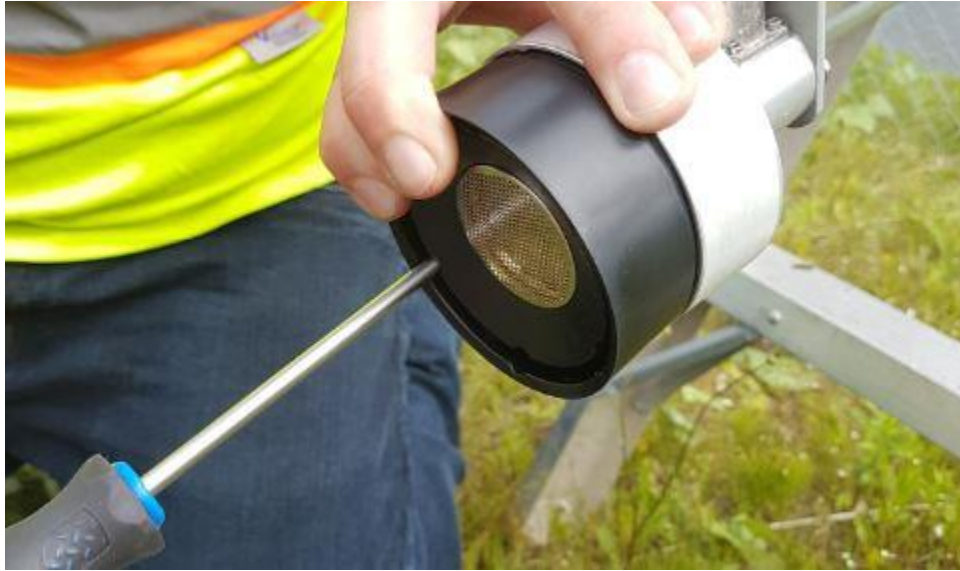
Figure 11: SR50 Screw Location
