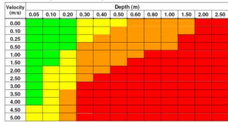
Figure 2: Flood Hazard Matrix (Uden et al, 2007)
