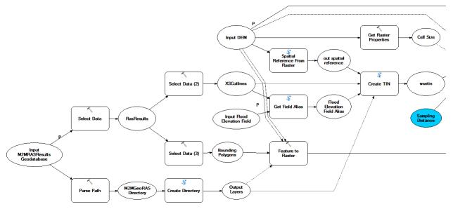
Figure 9. "GeoRAS to Flood" model details (1/2).
