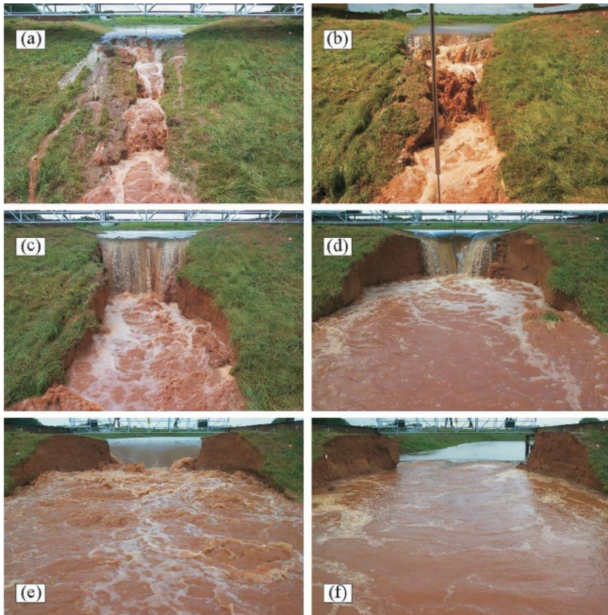
Figure 1: Stages of the erosion process that lead to the breaching of the earthen dam. (Wu, et al., 2011)
