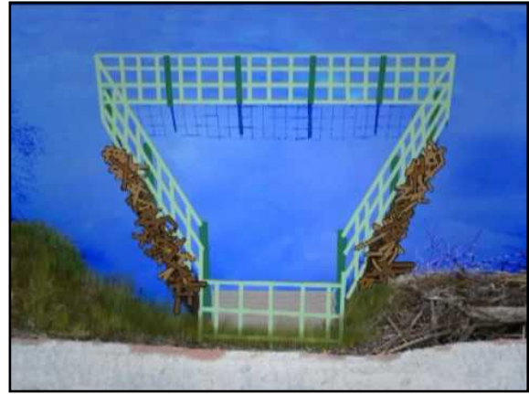
Figure 8 - Trapezoidal fencing around culvert to deter beaver damming. Culvert entrance at bottom of figure with debris caught by fencing. Image retrieved from Perryman, 2010.
