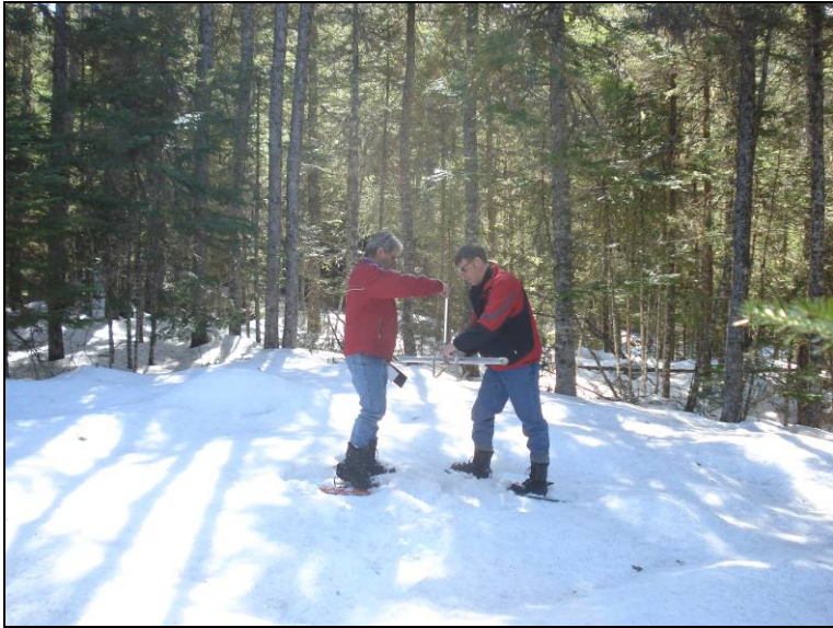
Figure 3. Jerry Smith (left) and Dawson Strangemore (right) of Deer Lake Power weight a snow sample at one of the Little Grand Lake (South) substations.
