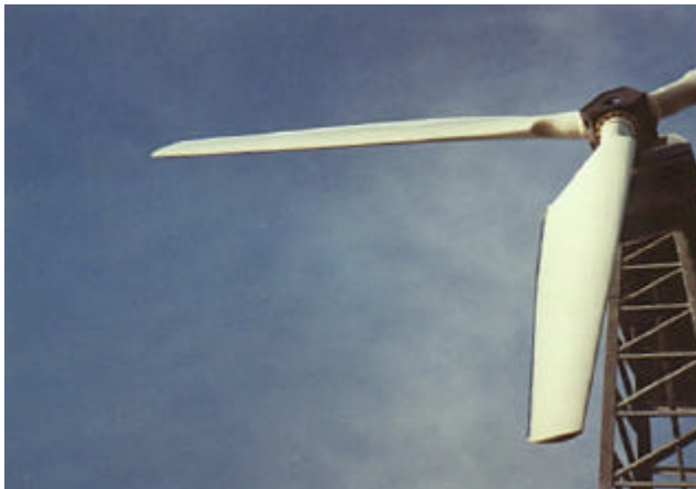
Figure 5 The fiberglass blades are rigidly connected to the hub. This fixed pitch design reduces costs and simplifies maintenance.
