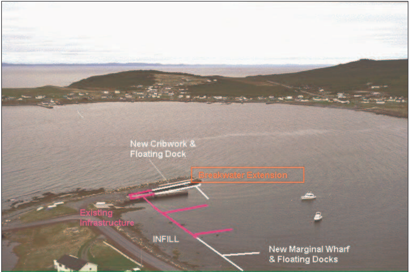
Figure 2: Photo showing the proposed developments for Phase II of Marina Development. Photo taken in 2000 before Phase I was completed.
