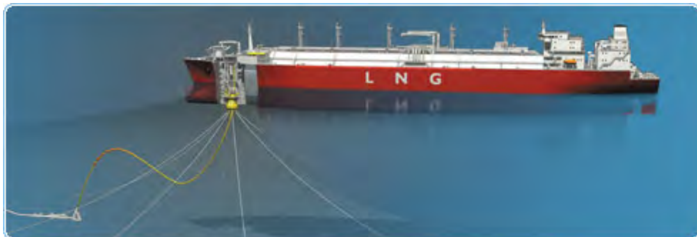
Figure 2.3 LNG Regasification Vessel with Submerged Turret Loading System
