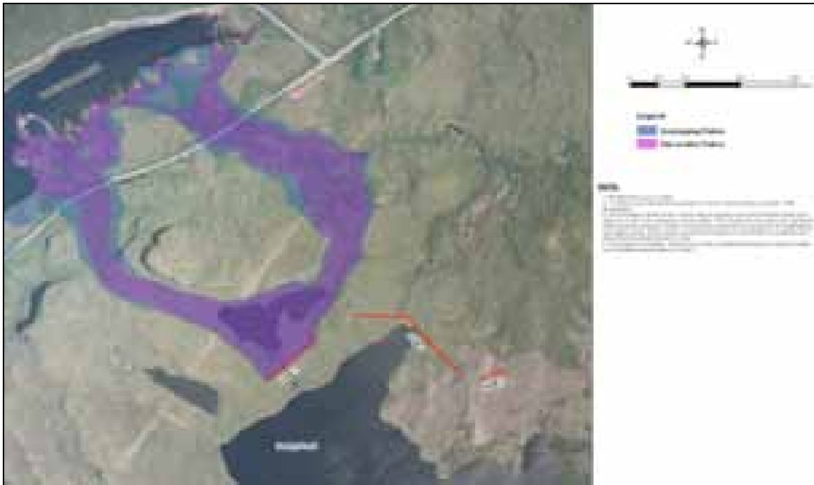
Figure 9.2 Sandy Pond Dam #1 Failure Flood Mapping
