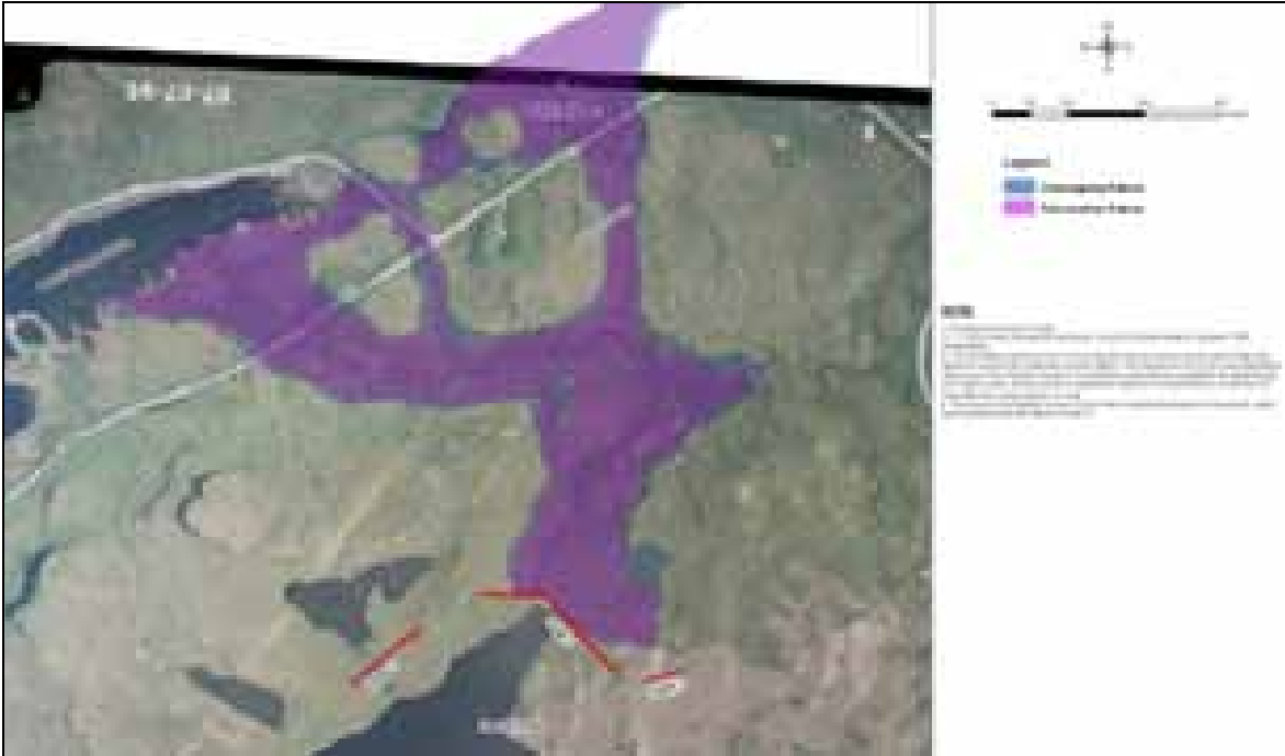
Figure 9.3 Sandy Pond Dam #2 Failure Flood Mapping
