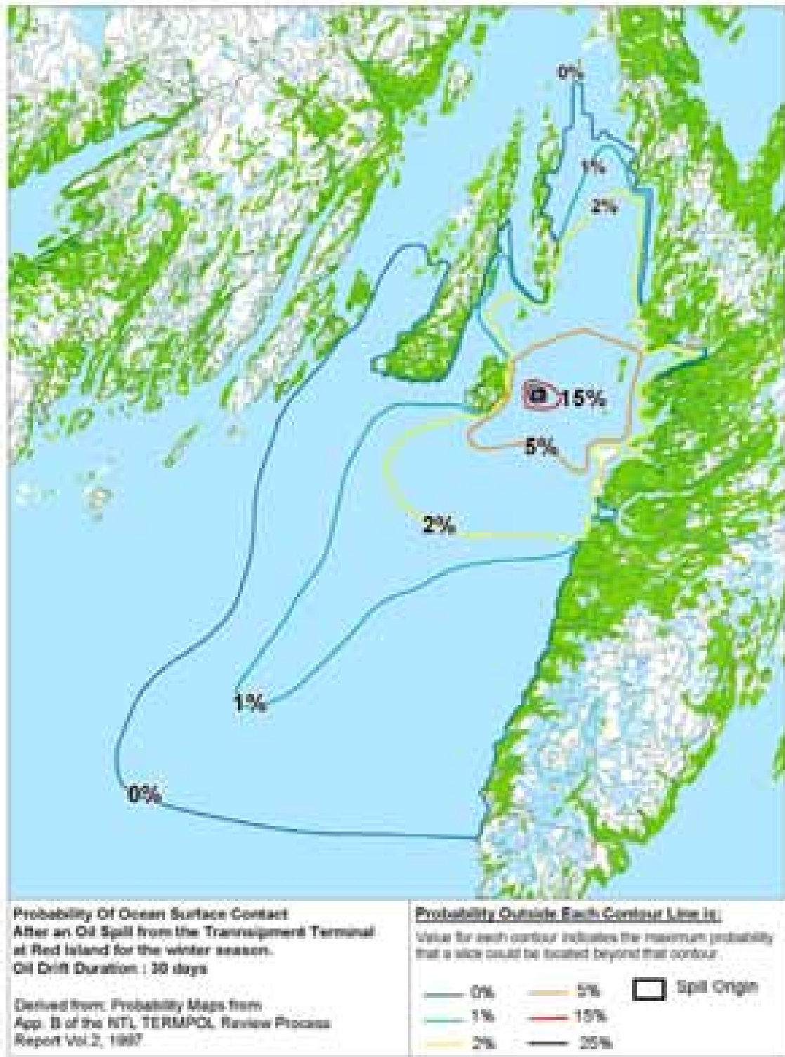
Figure 7.6 Probability of Ocean Surface Contact After an Oil Spill from the Transshipment Terminal at Red Island for the winter season
