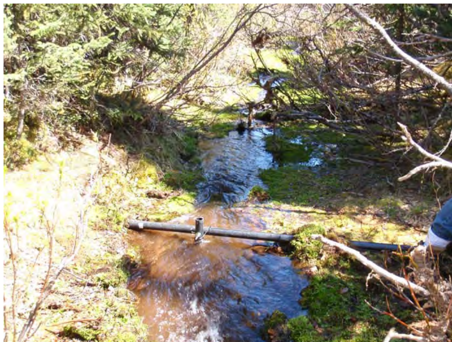
Photograph 1: SG2 Stream Gauge Levellogger Looking Southeast
