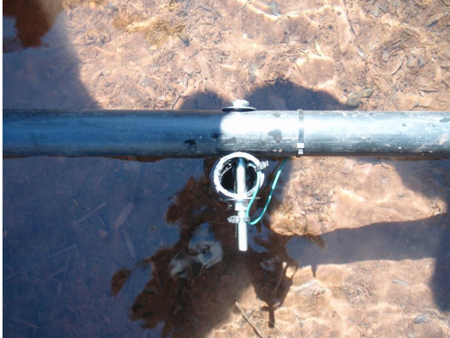
Figure 2 SG1 Stream Gauge Levellogger
