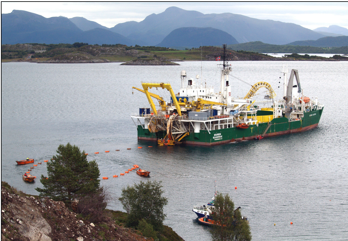
Figure 2.11 Typical Cable-Laying Vessel
