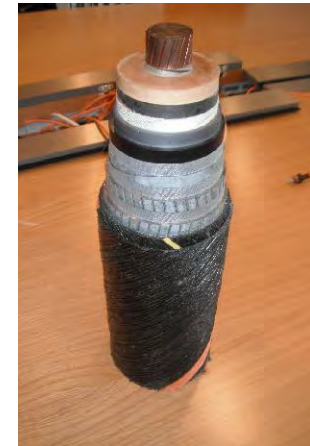
b) CROSS SECTION OF A TYPICAL SUBMARINE CABLE
