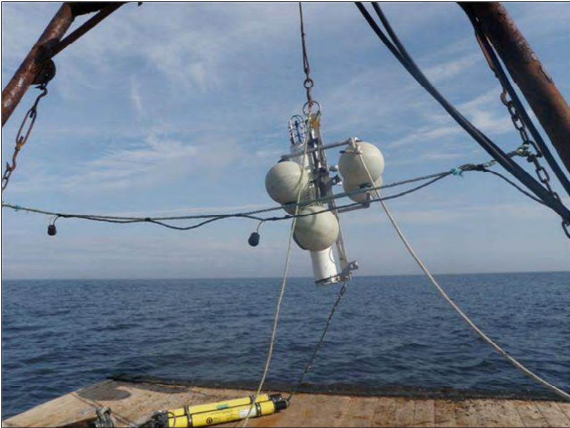
Figure 2.1 AURAL Recorder (white) on a float frame with dual acoustic releases (yellow) before deployment at the Newfoundland Station.
