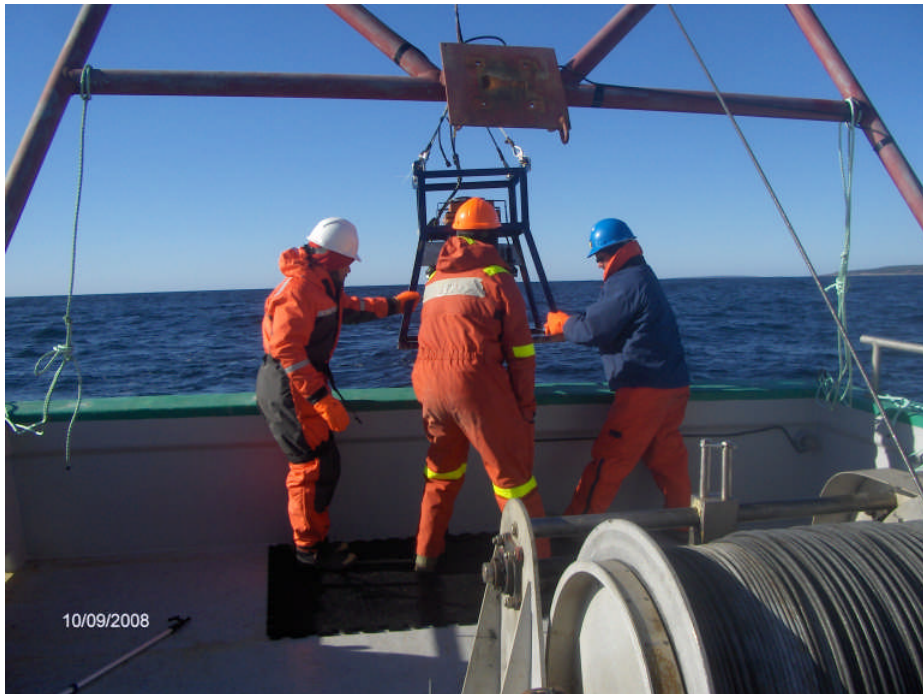
Photo B-4. Deploying the Drop Video (2008)
