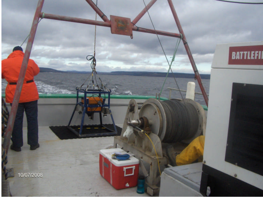
Photo B-3. Drop Video Attached to A-frame and Winch (2008)
