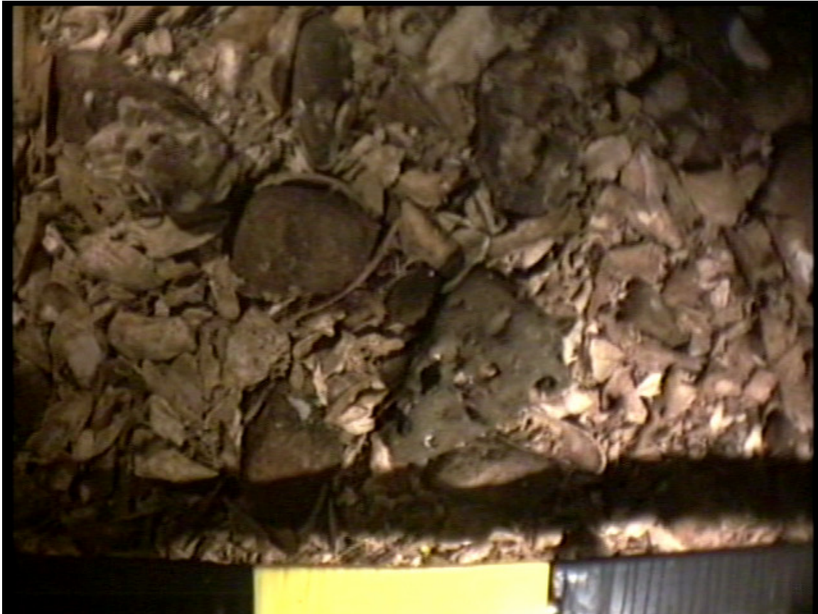
Figure 3.8. Mixed Coarse-Small / Shells substrate at approximately KP 4.8. Lithic fragments are larger in this region. Video frame grab from the 2008 survey by Amec (image is 30 cm wide).
