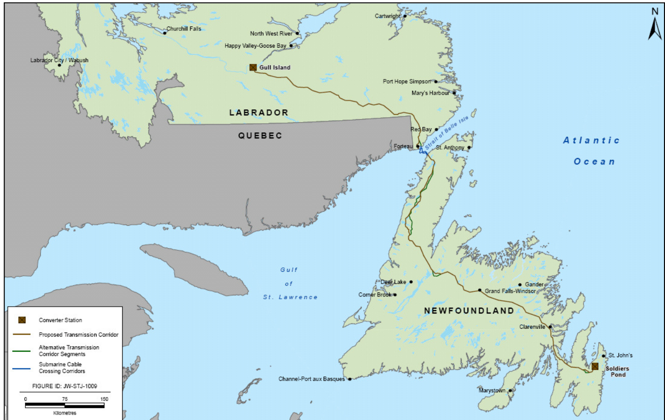
Figure 1.1. Labrador – Island Transmission Link: Project Overview
