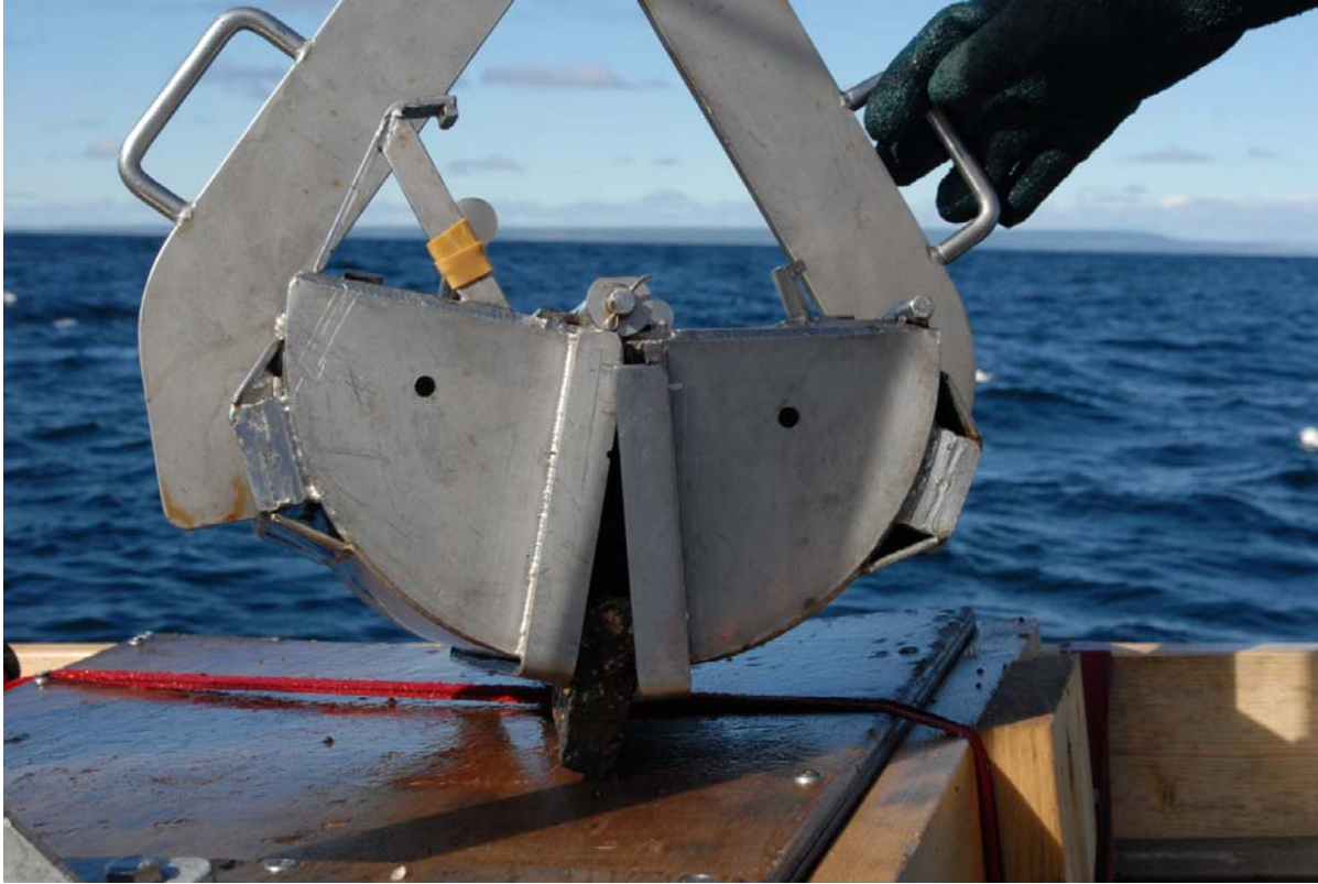
Figure 2.6 Van Veen Sediment Grab with Jaws Held Open by Large Substrate Material
