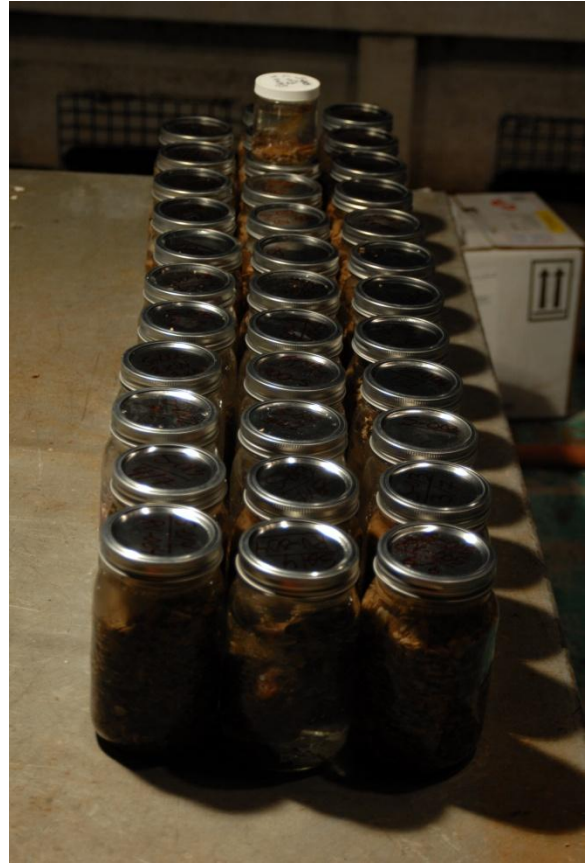
Figure C.12 Benthic samples preserved in 10% buffered formalin prior to shipment to the laboratory for analyses
