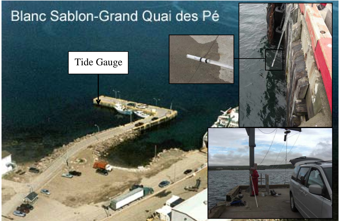
Figure 2.2-2: Installation and Retrieval of Nalcor Tidal Gauge at Blanc Sablon (background picture source: DFO List of Harbours and Harbour Authorities, 2009).
